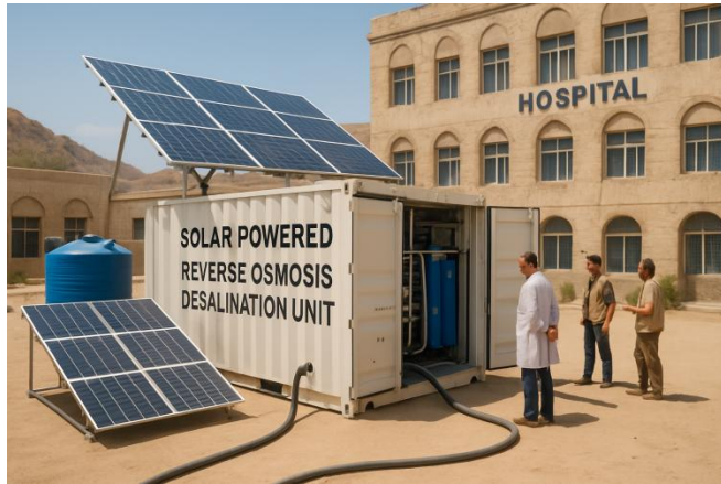
Fig. 10. A containerized solar RO unit with off-grid operation and small mobility, the rapid-response mobile desalination unit is designed for emergency deployment in areas affected by conflict.
