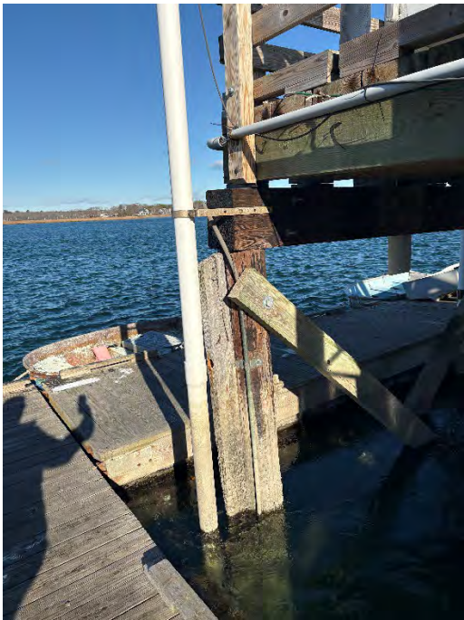
Photo 3: Stainless steel brackets help keep this PVC deployment tube away from dock pier and wharf pilings. WENRR's sonde is secured at the bottom of this tube.
