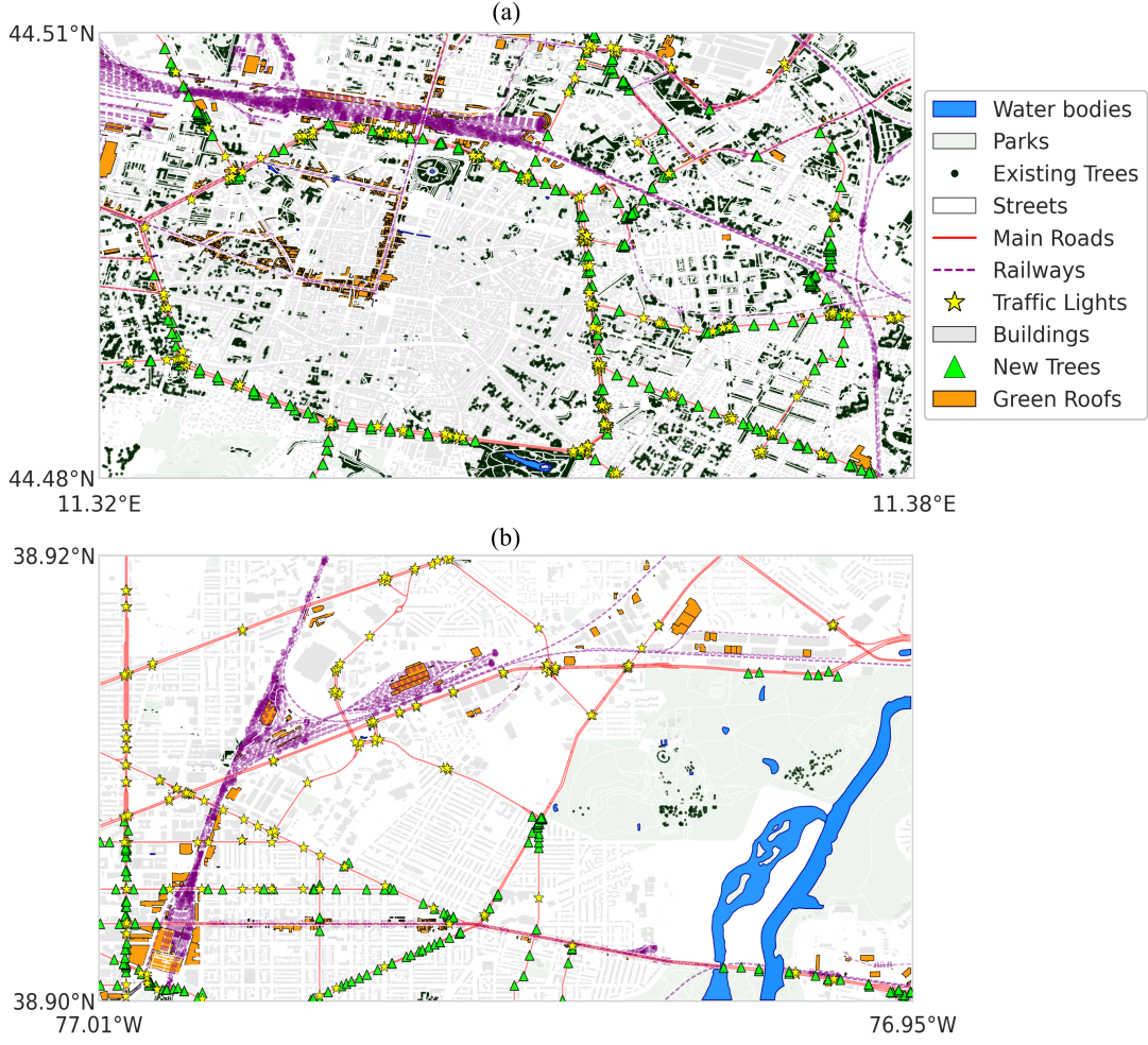
Fig. 17. Spatial implementation of urban greening: a) Bologna and b) Washington, D.C., showing new trees (green triangles) along main roads (red lines), green roofs (yellow squares) on buildings with \text{NDVI} \leq 0.2 near railways (dashed purple), and traffic lights (yellow stars).
