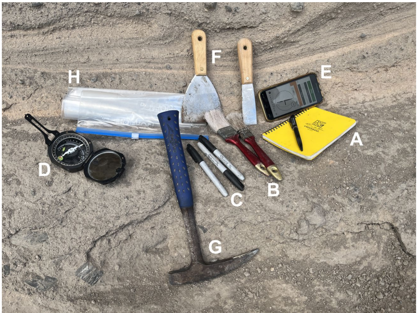
285 Figure 7: Key equipment for paleomagnetic sampling of pyroclastic deposits. [A] field notebook, [B] brushes of varying sizes for cleaning rock samples before labeling, [C] permanent markers for labeling, [D] example of a geological compass-clinometer for orienting samples, [E] example of a smartphone compass-clinometer app that can also be used for sample orientation, [F] metal spatulas of varying sizes for cleaning the outcrop and the samples, [G] geological hammer/pick for cleaning the area around the sample and removing the sample from the outcrop, [H] cloth and plastic sample bags for organizing oriented samples.
