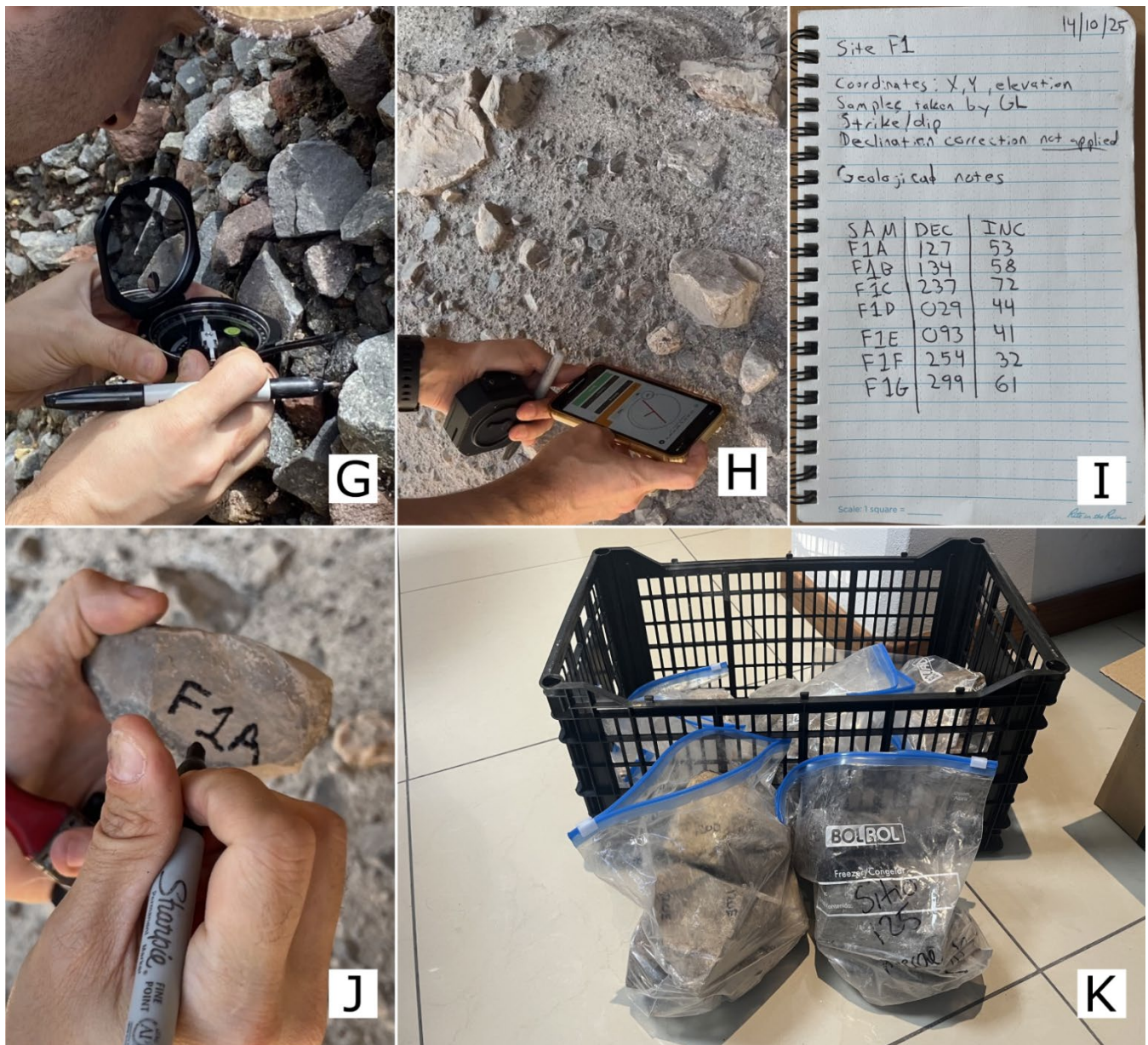
Figure 8: Steps for taking oriented paleomagnetic samples from a pyroclastic deposit outcrop. [A] example of a field notebook page prepared for notes on sampling and orientation, [B] examining the outcrop to choose ideal clasts for sampling, [C] example of an outcrop with a clast dipping away from the outcrop circled in red and an a clast with an inverted flat surface circled in blue, [D] cleaning the surface of a sample and clearing space around it before orientation and labelling, [E] using a permanent marker to draw a strike arrow parallel to the measurement being taken by the compass, [F] clast with the orientation arrow drawn for strike (indicated by red arrow) and tick mark for dip (indicted by smaller, black arrow), [G] measuring the declination of the sample with the geological compass, [H] measuring the declination and inclination of the flat sample face with a smartphone compass-clinometer app, [I] example of a standard field notebook table with sample names and orientations, [J]
