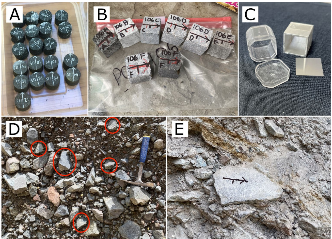
Figure 6: Photos showing important paleomagnetic sample and specimen characteristics. [A] example of 25 mm diameter, 25 mm-thick cylindrical rock specimens, [B] 2 x 2 x 2 mm rock cube specimens, [C] specialized plastic and metal boxes for collecting 2 x 2 x 2 cubic samples of matrix, [D] PDC outcrop with several viable hand samples highlighted, [E] example of an ideal hand sample, note the flat face of rock that is ideal for measuring and labeling.
