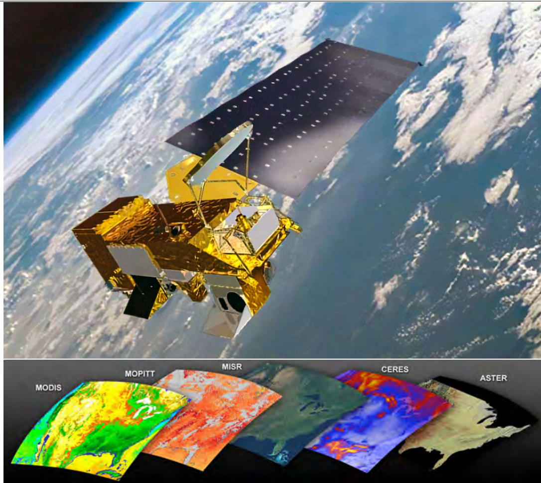
Figure 10.3: Terra Earth observatory satellite collects data about the Earth's bio-geochemical and energy systems using five sensors that observe the atmosphere, land surface, oceans, snow and ice, and the planetary energy budget. The five Terra onboard sensors are: ASTER (Advanced Spaceborne Thermal Emission and Reflection Radiometer) CERES (Clouds and Earth's Radiant Energy System) MISR (Multi-angle Imaging SpectroRadiometer) MODIS (Moderate-resolution Imaging Spectroradiometer) MOPITT (Measurements of Pollution in the Troposphere). Source: NASA – Terra , accessed 11/01/2024
