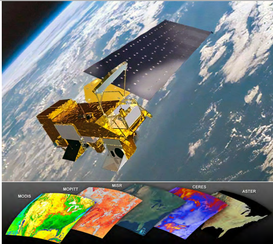
Figure 12.3: Terra Earth observatory satellite collects data about the Earth's bio-geochemical and energy systems using five sensors that observe the atmosphere, land surface, oceans, snow and ice, and the planetary energy budget. The five Terra onboard sensors are: ASTER (Advanced Spaceborne Thermal Emission and Reflection Radiometer) CERES (Clouds and Earth's Radiant Energy System) MISR (Multi-angle Imaging SpectroRadiometer) MODIS (Moderate-resolution Imaging Spectroradiometer) MOPITT (Measurements of Pollution in the Troposphere). Source: NASA – Terra , accessed 11/01/2024
