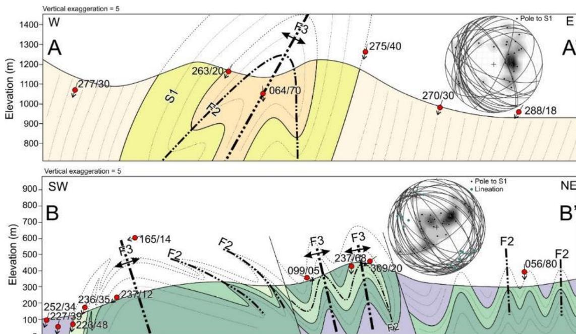
323 Figure 6 Geological cross-sections of transects labelled in Figure 5. Sections generated using QProf
