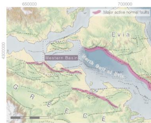
The Kalypso Fault: Major offshore syn-kinematic normal fault zone
