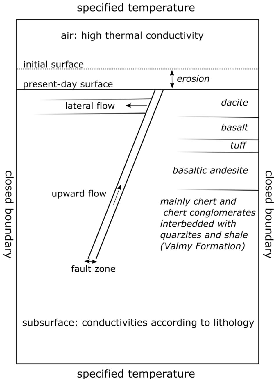
**Figure DR2** Schematic diagram depicting the hydrostratigraphic framework model of the discharge area of the Beowawe hydrothermal system. The upper and lower boundary conditions were assigned a specified temperature according to the average annual air temperature and the regional geothermal gradient. No heat flow is allowed over the left and right hand model boundary. Fluid flows upwards along a single fault zone, part of the flux
