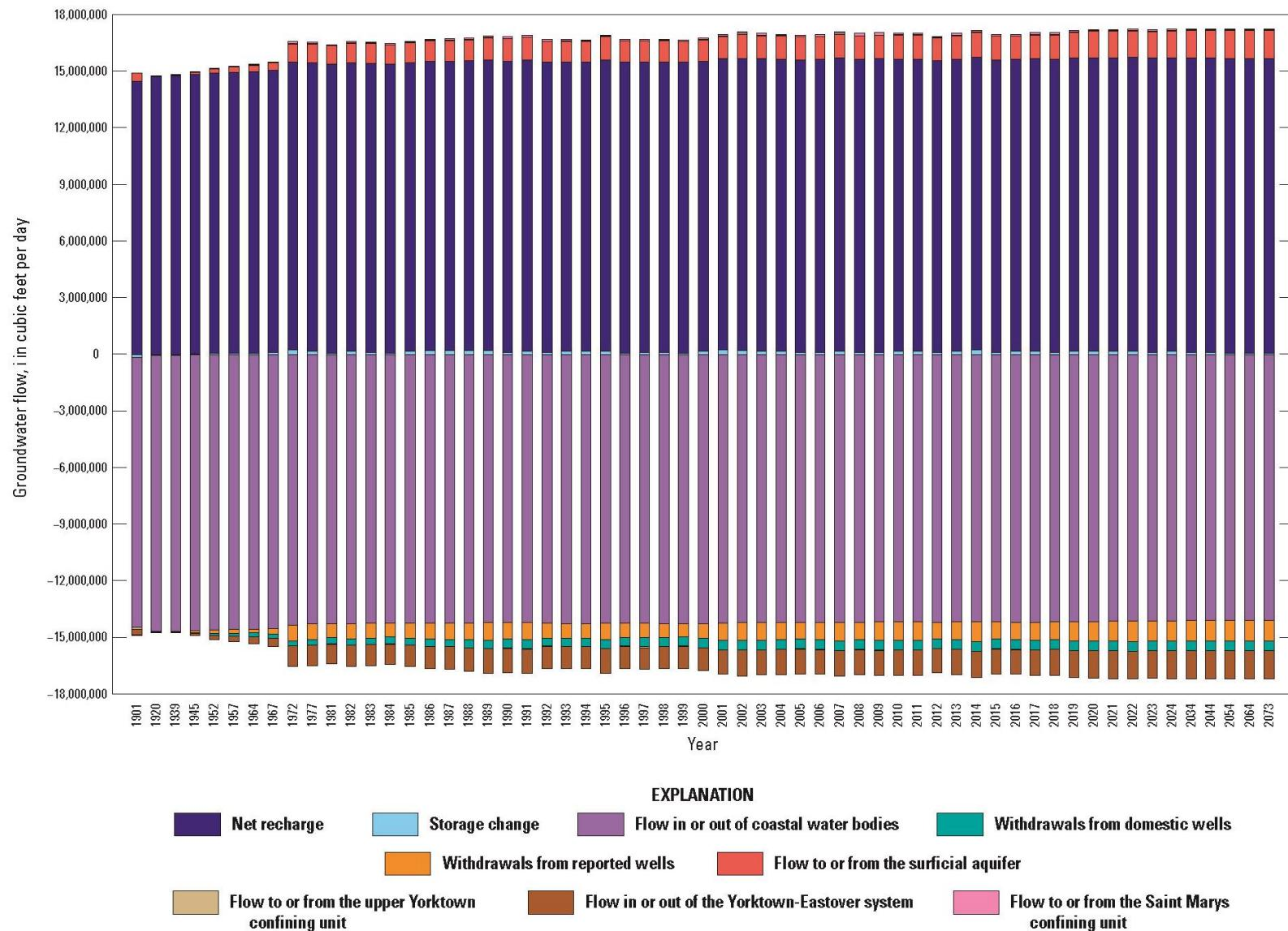
**Figure 11.** Simulated groundwater budgets for the entire Virginia Eastern Shore model area for all model periods. Historical and future periods are multiple years in length. Groundwater flow values are in cubic feet per day.
