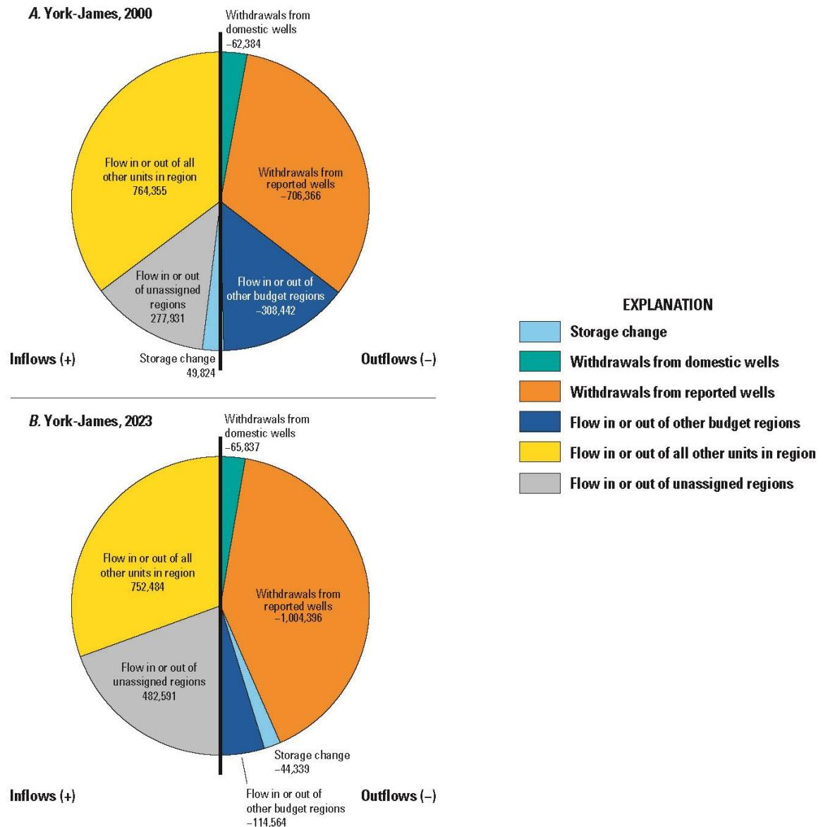
**Figure 21.** Simulated yearly groundwater budgets for the Potomac aquifer in the York-James region of the Virginia Coastal Plain for the years A, 2000, and B, 2023. Groundwater flow values are in cubic feet per day.
