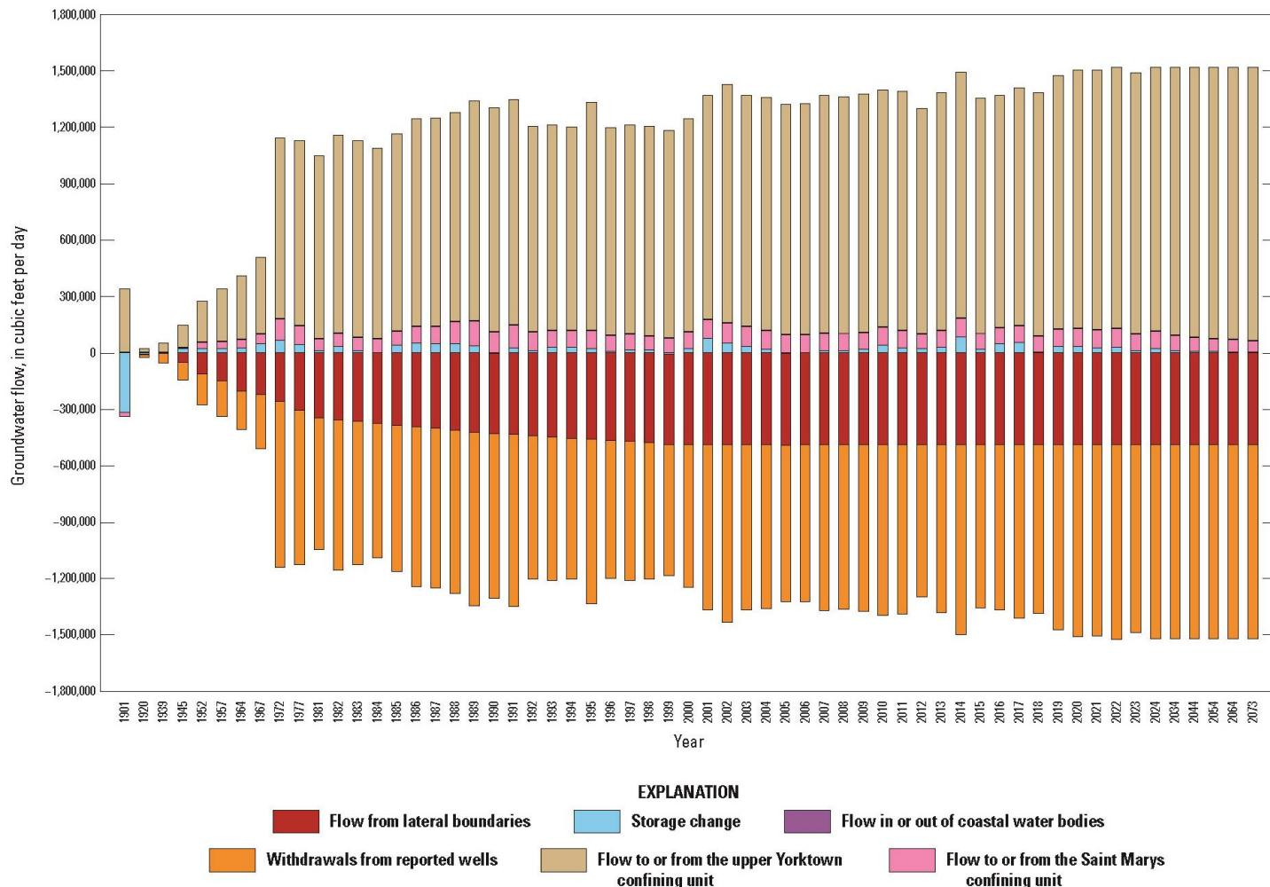
**Figure 28.** Simulated groundwater budgets for the combined Yorktown-Eastover aquifer system in the Virginia Eastern Shore model for all model time periods. Time periods for historical and future periods are multiple years in length. Groundwater flow values are in cubic feet per day.
