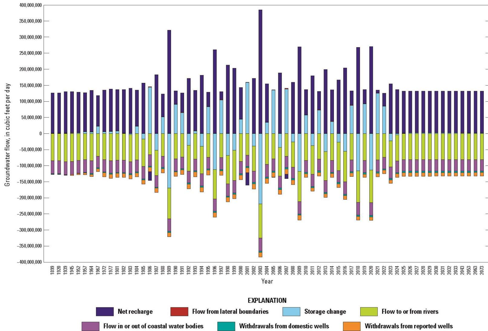
**Figure 8.** Simulated groundwater budgets for the entire Virginia Coastal Plain model area for all model periods, illustrating budget components. Historical and future periods are multiple years in length.
