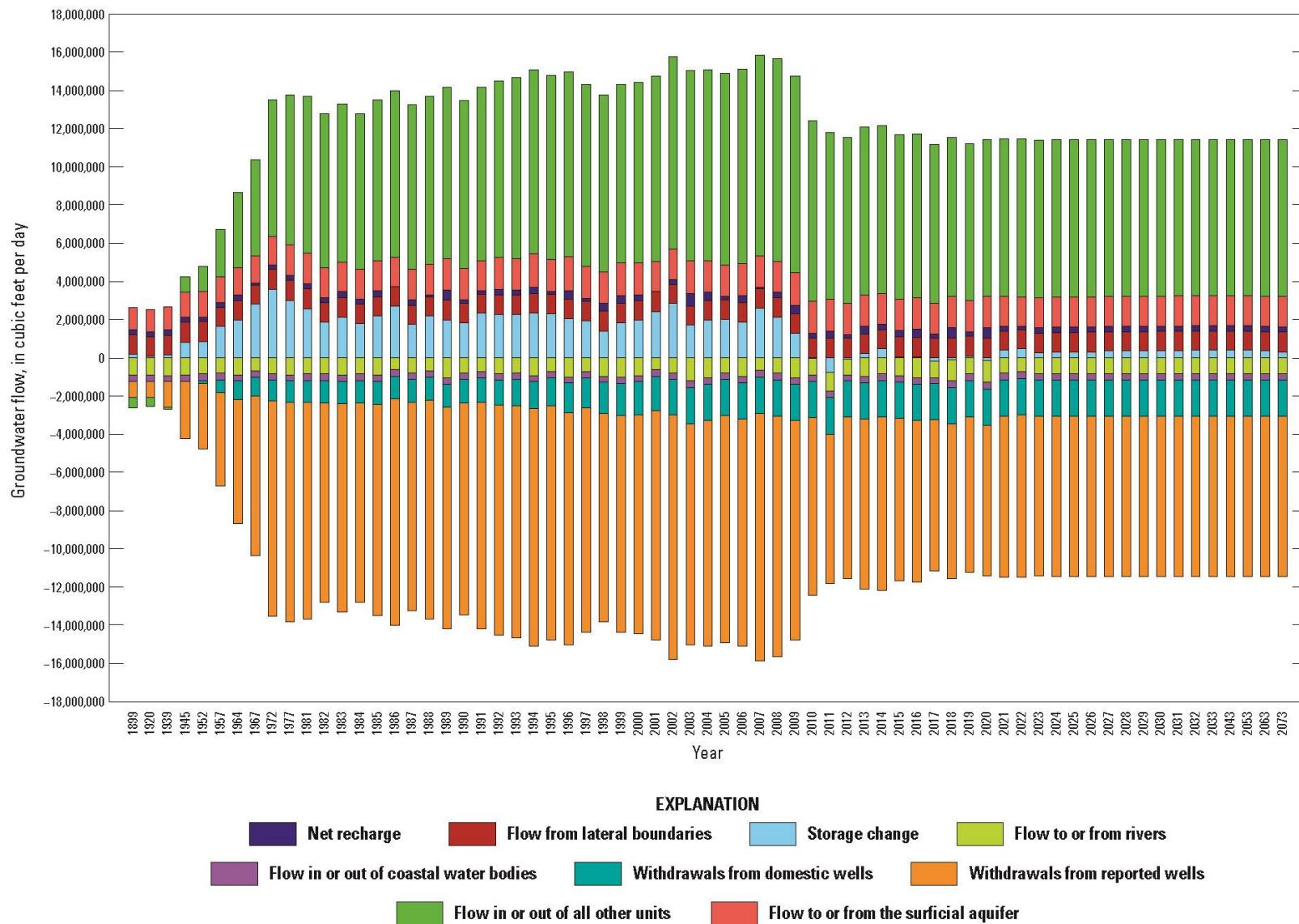
**Figure 10.** Simulated groundwater budgets for the entire Virginia Coastal Plain model area for all model periods for the Potomac aquifer in the Virginia Coastal Plain model. Historical and future periods are multiple years in length. Groundwater flow values are in cubic feet per day.
