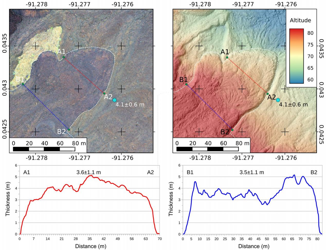
439 Figure 7. High resolution orthomosaic and digital surface model and corresponding topographic
