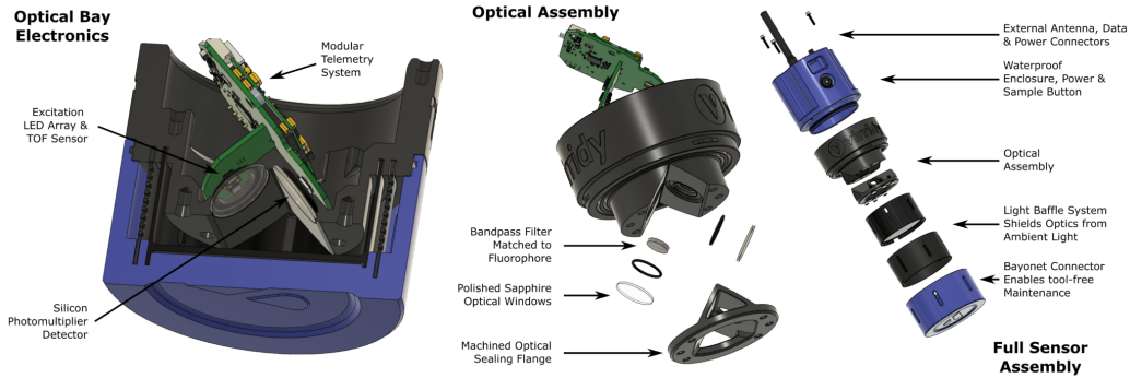
Figure 2: Fluorimeter mechanical, electrical and optical assembly.
