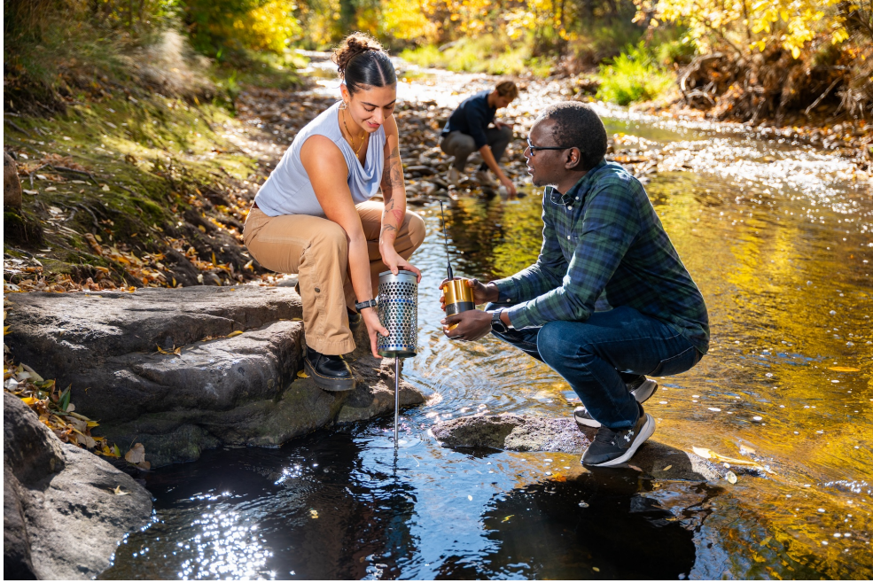
Figure 1: The fluorimeter technology deployed in Boulder Creek, Colorado. A typical installation includes the fluoroimeter (at right in gold), an enclosure anchored on the shore (left), a wired antenna if the unit is fully submerged, and complemented by sampling and enumeration (center).
