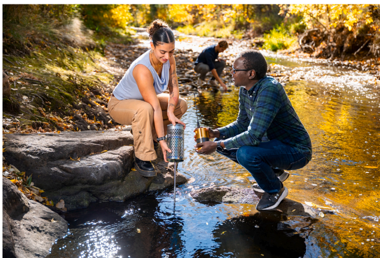
Fig. 1. The fluorimeter technology deployed in Boulder Creek, Colorado. A typical installation includes the fluorimeter (at right in gold), an enclosure anchored on the shore (left), a wired antenna if the unit is fully submerged, and complemented by sampling and enumeration (center). Photograph is unedited; individuals pictured provided consent for publication. (For interpretation of the references to color in this figure legend, the reader is referred to the web version of this article.)
