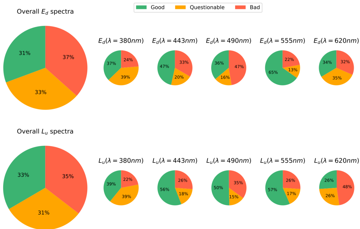
Fig. 6. Distribution of E_d profile (upper panel) and L_u profile (lower panel) types for each wavelength and for the overall hyperspectral profile.
