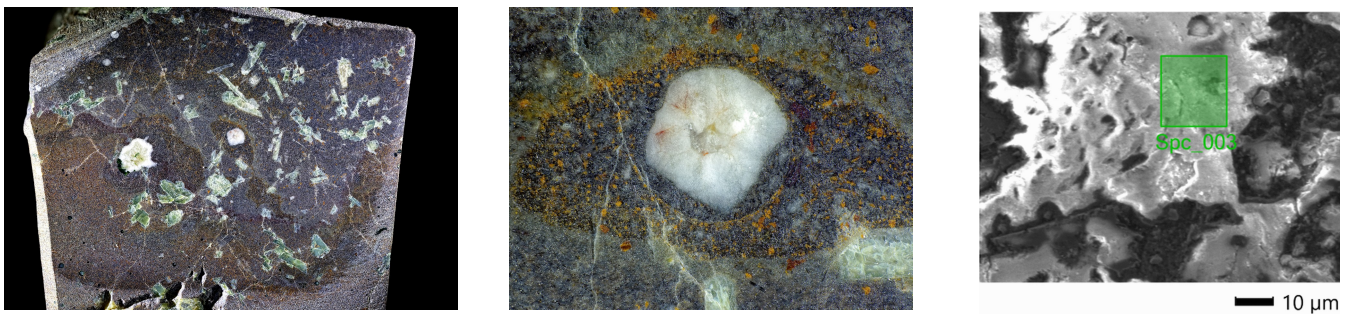
Figure 12: Petrographic analysis of sample 4. Left: Polished section (approx. 5 cm width). Middle: Detailed micrograph of the reaction textures. The dark matrix hosts large plagioclase phenocrysts, finely dispersed brown analcime, and acicular clinopyroxene. The prominent white, rounded domains are products of the autometasomatic, post-magmatic evolution in a closed system. These domains predominantly consist of calcite, montmorillonite, and natrolite. The reaction front is clearly discernible. Within this zone, analcime has been almost entirely consumed, reacting with plagioclase to form the secondary assemblage. Plagioclase crystals outside this reaction zone remain pristine and unaffected by the carbonation process. Photos: Matthias Hanke Collection. Right: SEM image of a carbonated plagioclase.
