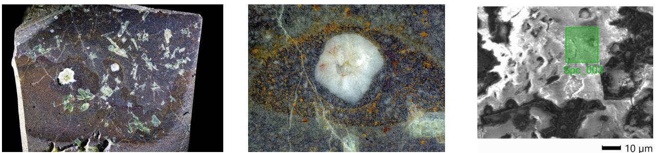
Figure 12: Petrographic analysis of sample 4. Left: Polished section (approx. 5 cm width). Middle: Detailed micrograph of the reaction textures. The dark matrix hosts large plagioclase phenocrysts, finely dispersed brown analcime, and acicular clinopyroxene. The prominent white, rounded domains are products of the autometamorphic, post-magmatic evolution in a closed system. These domains predominantly consist of calcite, montmorillonite, and natrolite. The reaction front is clearly discernible. Within this zone, analcime has been almost entirely consumed, reacting with plagioclase to form the secondary assemblage. Plagioclase crystals outside this reaction zone remain pristine and unaffected by the carbonation process. Photos: Matthias Hanke Collection. Right: SEM image of a carbonated plagioklas.
