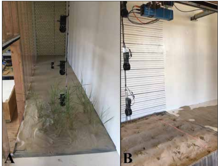
Figure 2. Inside the wind tunnel chamber. (A) Pre-experiment, a 1 m x 1 m x 0.3 m box is sealed into the test area level with the 3.6m-long upwind chamber bed. Prior to trials the bed and box are leveled to a 1-inch (2.54 cm) uniform height. Here the upwind bed has been leveled, but the box has not yet been leveled. Turbulence is reduced as the air is pulled through the honeycomb wall into the chamber and towards the plants. The four black sensors are moveable anemometers. The three vertical anemometers provide a wind profile in the test area among the plants, and there is also an anemometer upwind and downwind (cannot be seen in the photo) of the test area. (B) Post-experiment, all above-ground plant material has been cut from surface using shop shears. Only plant parts too close to the surface to cut without disturbing the bedforms remain. The 3D sensor is mounted on a track that has been lowered toward the bed from the ceiling for data acquisition. The 3D sensor is mechanically pulled over the test area to scan the topography with the red laser denoting the area the sensor is currently passing over.
