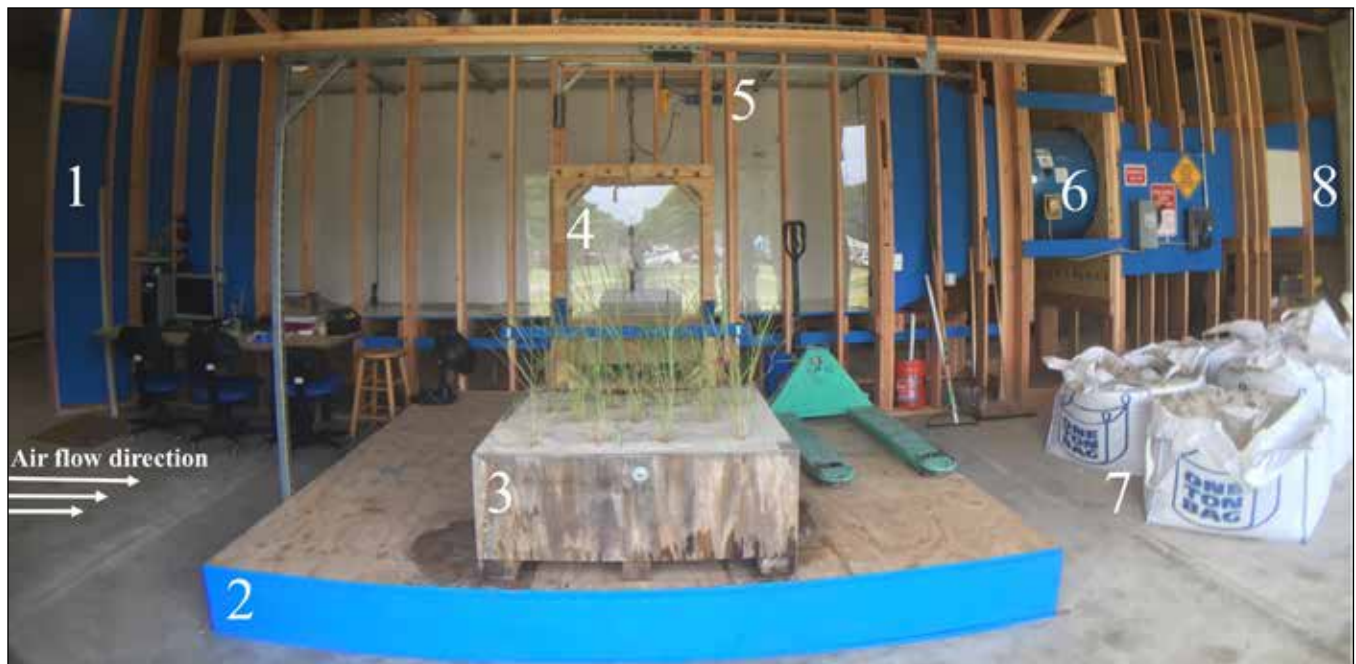
Figure 1. Movable bed wind tunnel built in Waretown, NJ, with USGS and ERDC funding in 2016. The wind tunnel is capable of reaching wind speeds up to 27 mph (12.1 m/s) and was designed with ease of use and adaptability in mind for future research applications. The main components are labeled numerically from left to right: (1) air flow inlet; (2) platform to insert boxes into test area; (3) one of the 1 m x 1 m x 0.3 m boxes in which we established our Ammophila plants; (4) test area where boxes are inserted and sealed into the chamber; (5) 3D sensor and accompanying hardware and tracking; (6) fan; (7) one ton bags of dry sand; and (8) air outflow.
