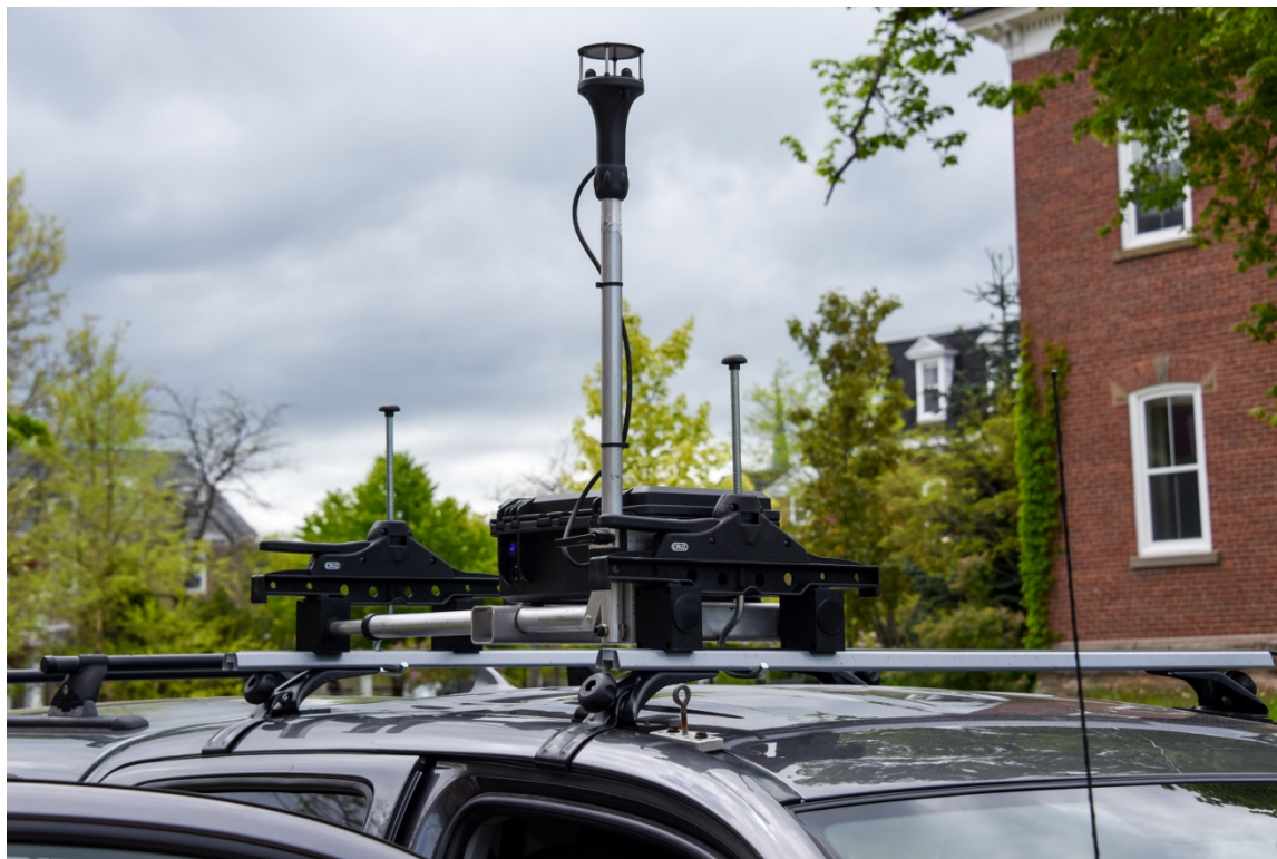
118 Figure 1. Rooftop-mounted vehicle-based measurement system.
