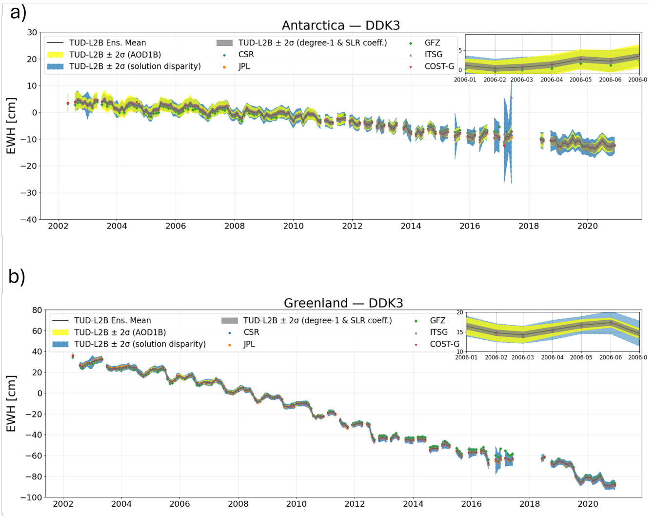
Figure 9. Land-averaged equivalent water height (EWH) time series for (a) Antarctica and (b) Greenland, derived from selected individual Level-2 GRACE/GRACE-FO DDK3-filtered solutions (CSR, JPL, GFZ, ITSG, and COST-G) and compared with the TUD ensemble mean (degree and order 2–60). Shaded envelopes indicate \pm 2\sigma (95%) uncertainty contributions associated with ensemble uncertainty, AOD1B de-aliasing, and the combined low-degree (degree-1 and SLR) uncertainty.
