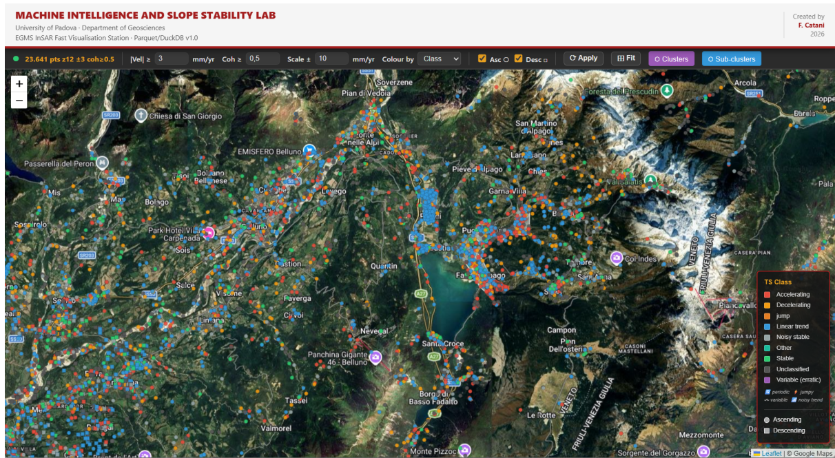
Figure 5: The MISSlab EGMS web viewer showing a portion of the Belluno–Alpago area (NE Italy, Veneto/Friuli-Venezia Giulia border). Points are coloured by time series class (legend, lower right); ascending-orbit points (Sentinel-1 tracks 015–139) are shown as circles and descending-orbit points (tracks 146–168) as squares. The viewer is displaying 23,641 points at zoom level 12 with |v| \geq 3 \text{ mm yr}^{-1} and coherence \geq 0.5 filters applied; the status bar (top left) shows the current filter state. The toolbar provides controls for velocity/class colour mode, coherence threshold, velocity scale, orbit selection, and cluster/sub-cluster polygon overlay. The viewer supports sub-100 ms viewport queries over the full \approx 300 M-point northern Italy database via the DuckDB/Flask bridge, enabling real-time interactive exploration comparable to a desktop GIS but without data subsampling.
