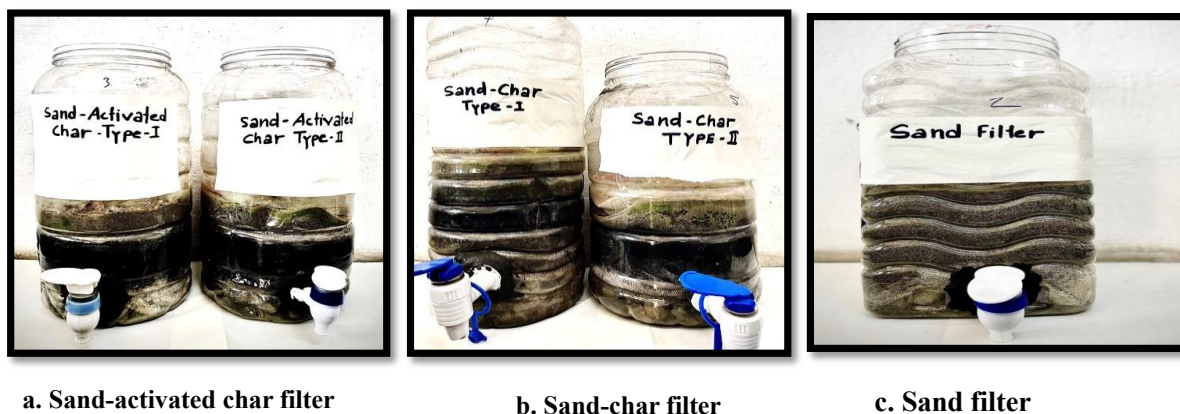
Figure 7. Low-cost filter models for microplastics filtration: a. sand-activated char filter, b. sand-char filter, and c. sand filter.
