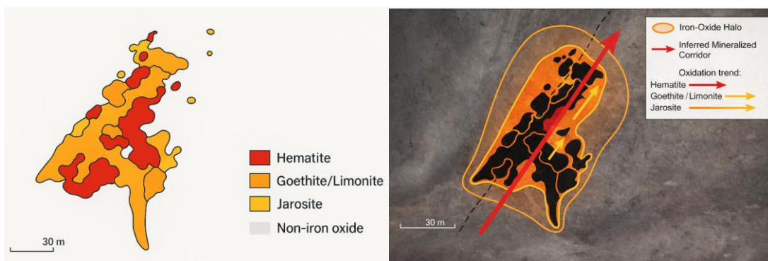
Figure 9. Left: simplified classification of iron-oxide surface expressions derived from HSV-transformed RGB imagery, highlighting the relative distributions of hematite, goethite/limonite, and jarosite within the target area. Right: interpretive overlay illustrating how these spectral proxies can be translated into a structurally coherent mineralization model, including delineation of the iron-oxide halo and inferred mineralized corridor. Dark patches in the right panel represent surficial excavation sites related to artisanal workings. The left panel represents the analytical classification, whereas the right panel demonstrates how the same image-derived information can be reorganized for target prioritization in a low-data exploration context. Source imagery: Google Earth / Google Earth Pro; Pléiades imagery © CNES/Airbus DS. HSV classification, interpretive overlay, and annotations by the authors.
