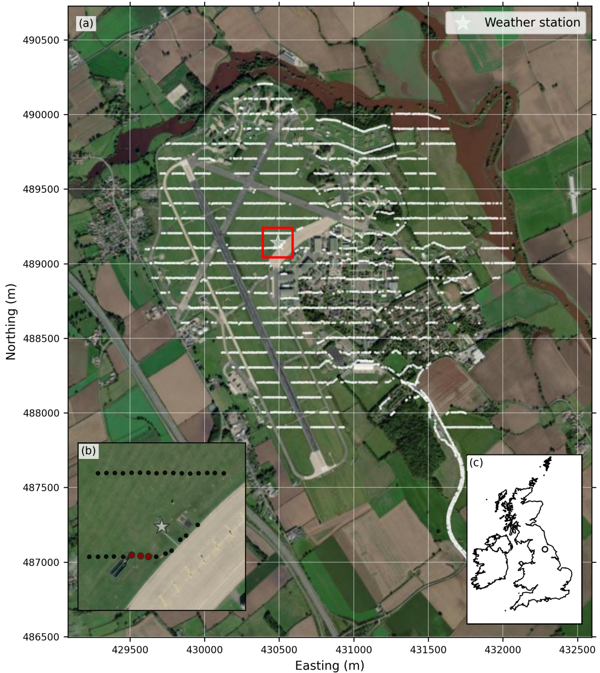
Figure 1. Location of the dense seismic array deployed at RAF Leeming, North Yorkshire, UK. (a) Location of 3,083 seismic nodes across the study area overlaid on aerial imagery (sourced from ESRI). The weather station used for calibration and comparison is indicated by the white star, while the red rectangle denotes the area shown in panel (b). (b) Detailed view of the sensor array surrounding the weather station, including the three calibration sensors (red symbols) used to develop the temperature bias-correction model. (c) Location of the study area within the United Kingdom. Coordinates are shown in the British National Grid
