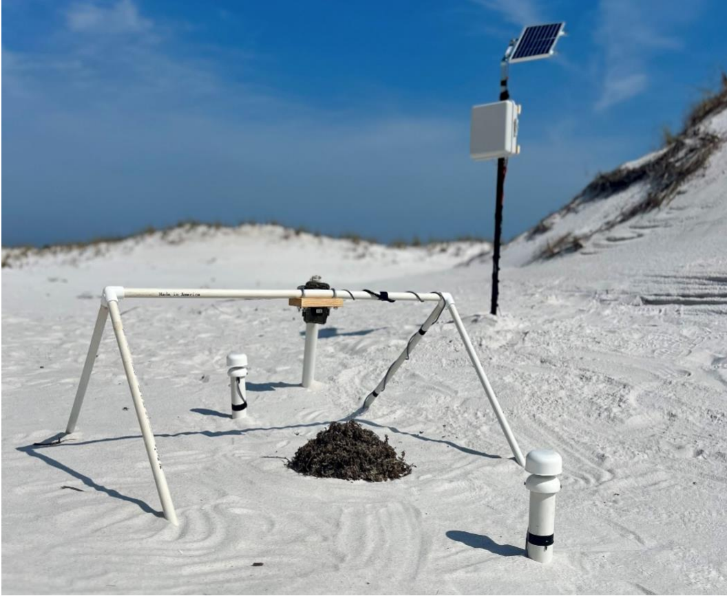
Figure 1 – Picture of field experiment setup showing 2D anemometers upwind and downwind of wrack pile along with single-point LiDAR.
