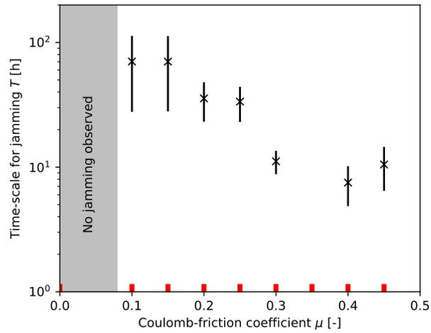
411 **Figure 8.** The influence of the Coulomb-frictional coefficient  $\mu$  (Eq. 10) on the characteristic time for
