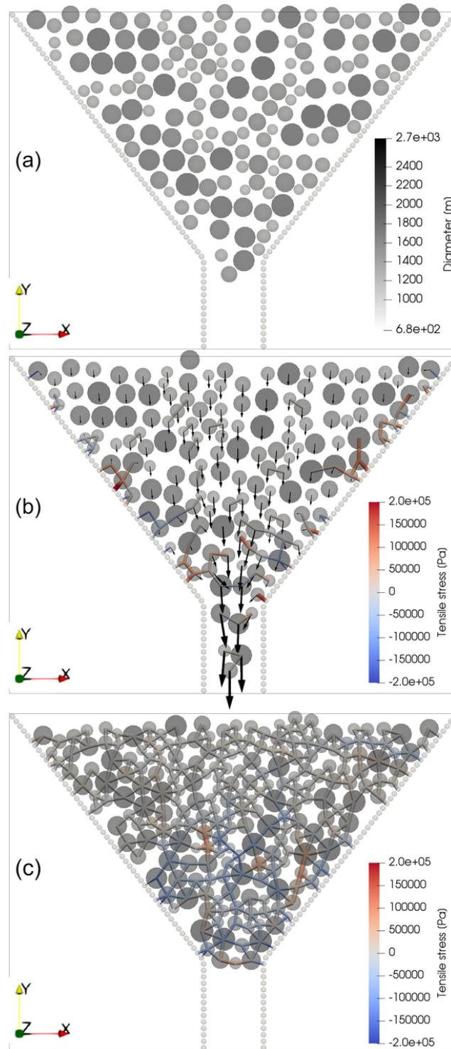
391 **Figure 5.** Example visualization of the granular system for the *idealized strait* runs, here the initial state (a),
