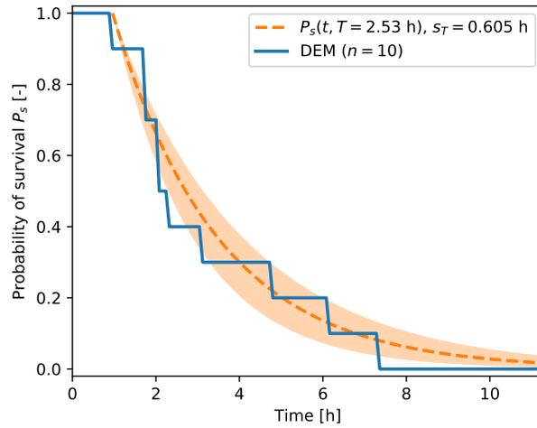
398 **Figure 7.** Probability of survival (non-jamming)  $P_s$  for the ensemble in Fig. 6, with a corresponding least-
