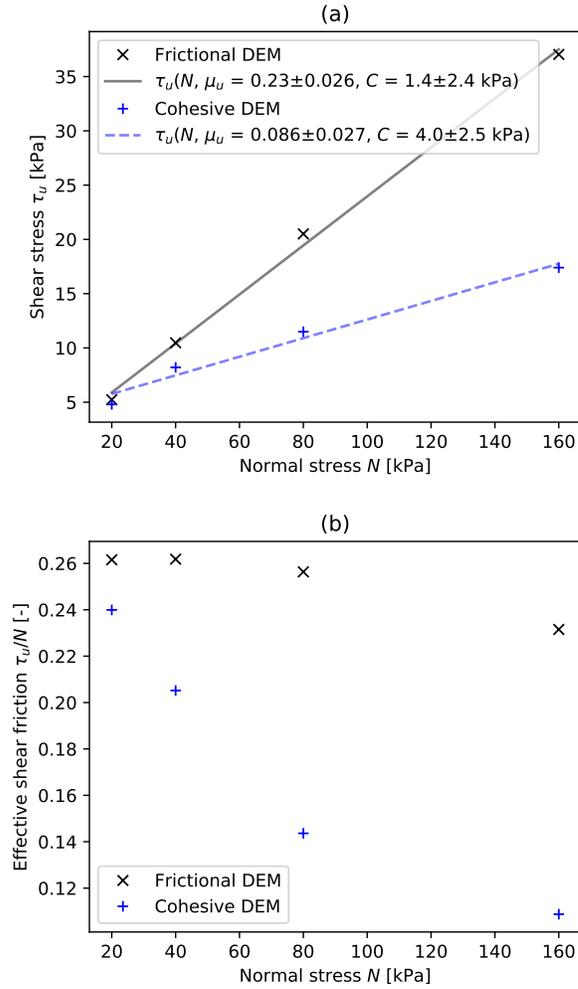
364 **Figure 3.** Steady-state stress and friction during simple shear for Coulomb-frictional model runs ( $\mu = 0.3$
