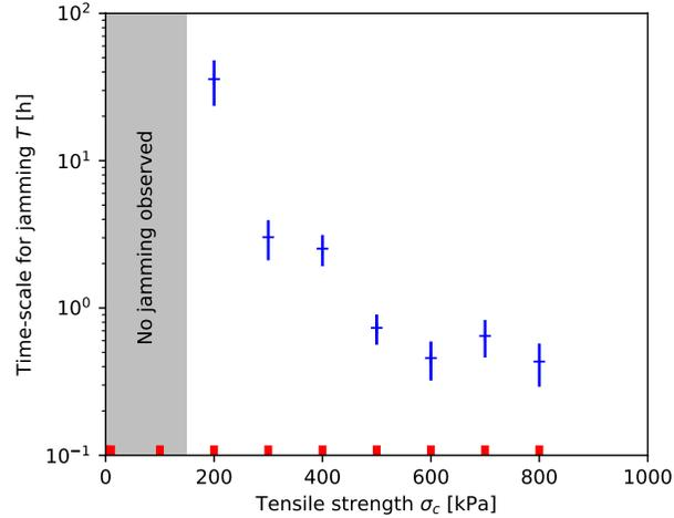
414 **Figure 9.** The influence of the tensile strength  $\sigma_c$  (Eq. 11) on the characteristic time for jamming  $T$  (Eq. 1)
