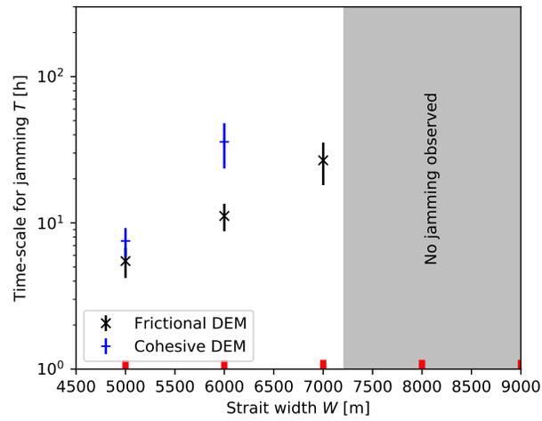
427 **Figure 10.** Jamming behavior with increasing width of the strait (Fig. 5) for Coulomb-frictional ( $\mu = 0.3$
