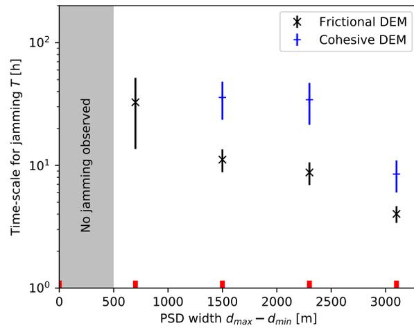
444 **Figure 11.** Jamming behavior with increasing width of the particle-size distribution for Coulomb-frictional
