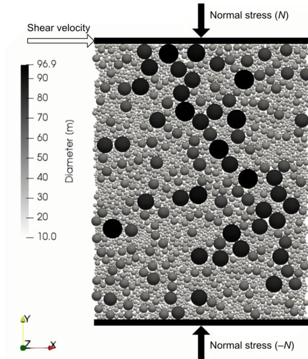
314 **Figure 1.** Simulation setup for the simple shear experiments. The upper and lower walls exert a prescribed
