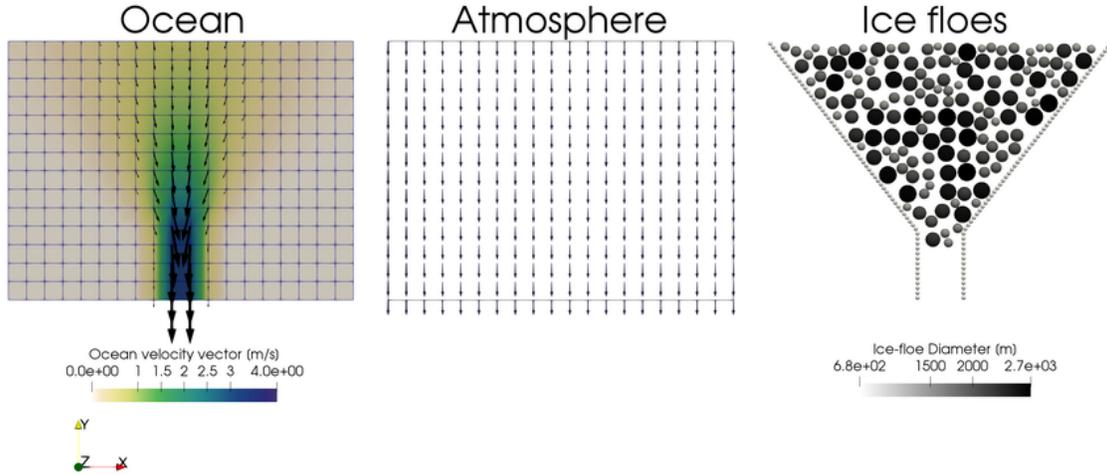
346 **Figure 2.** Simulation setup for the idealized strait experiments. Ocean velocities vary from 0 to 4 m/s
