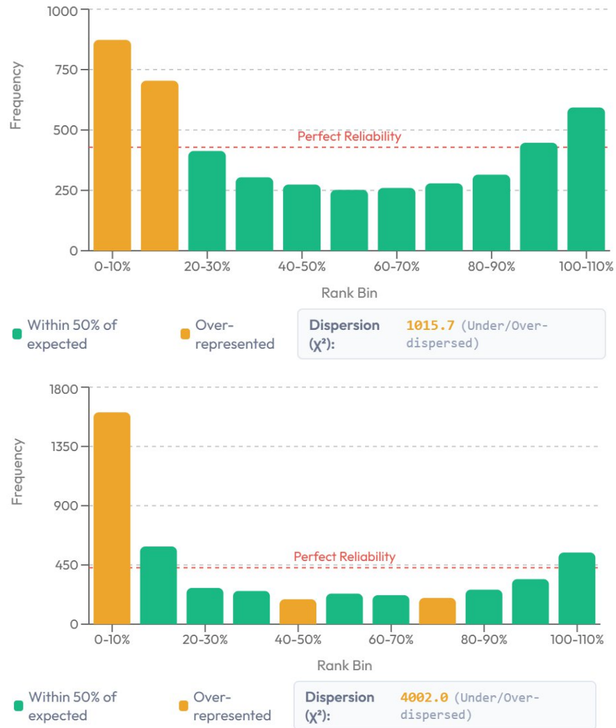
Figure 6. Reliability diagrams showing rank histogram distributions comparing observed streamflow against ensemble predictions from (a) NWM v2.1 (top) and (b) NWM v3.0 (bottom). Each bar represents the frequency of observations falling within a given rank bin (0–10% through 100–110%) across the ensemble; a perfectly reliable ensemble produces a uniform distribution matching the red dashed reference line ("Perfect Reliability"). Bars shaded orange indicate over-represented bins (frequency exceeding 50% above expected), reflecting systematic ensemble under-dispersion or directional bias at those ranks; green bars fall within 50% of the expected uniform frequency. The dispersion statistic ( \chi^2 ) quantifies overall departure from uniformity — larger values indicate greater unreliability; values of 1015.7 (v2.1) and 4002.0 (v3.0) both indicate significant over-dispersion (Under/Over-dispersed), with the pronounced spike at the 0–10% rank bin in both panels reflecting persistent ensemble over-prediction relative to observations.
