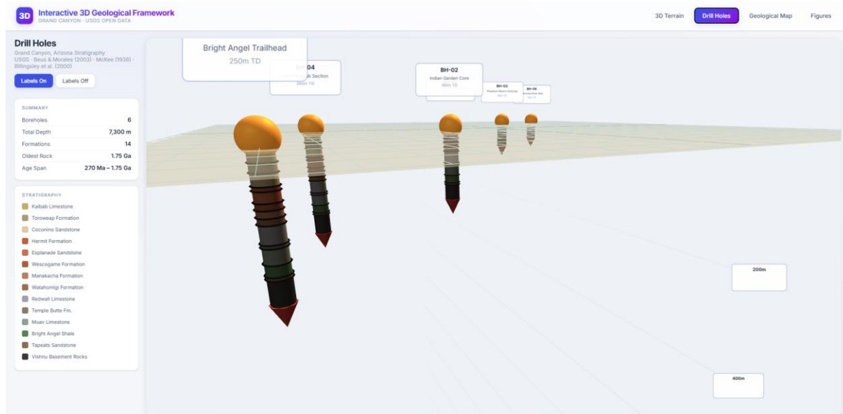
Figure 3. Close-up view of the 3D stratigraphic borehole module in action
