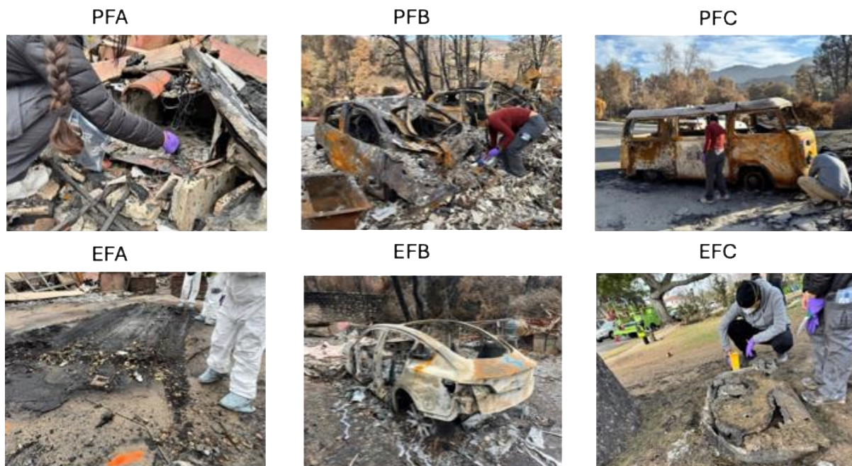
Figure S4. Collection of burned source materials from fire-impacted structures and vehicles following the 2025 Los Angeles fires. EFD is not shown. General characteristics of the samples are provided in Table S1.
