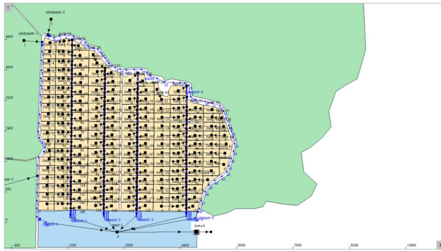
Fig.20. Connection state between catchment, channeling ditch, paddy field, drainage channel, regulation pond and drainage gate
