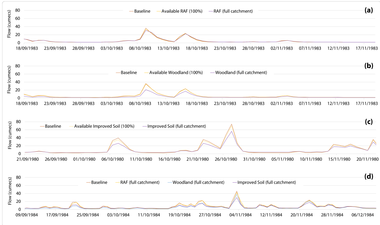
Figure S2: Sensitivity analysis comparing baseline, 100 percent grid-cells of maximum available, and hypothetical whole-catchment NFM hydrographs at the catchment outlet for (a) RAFs, (b) woodland, and (c) improved soil across representative short periods, and (d) whole-catchment comparison of all three NFM types.
