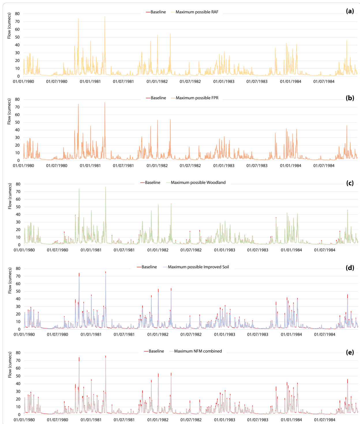
Figure S1: Simulated baseline and maximum NFM hydrographs at the catchment outlet over the five-year period (1980–1984) for (a) RAFs, (b) floodplain reconnection, (c) woodland, (d) improved soil, and (e) all NFM combined, illustrating the peak flow attenuation achieved by each intervention type at its maximum available extent.
