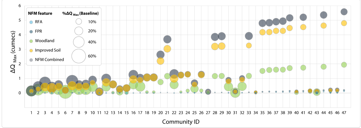
Figure 10: Maximum flow reduction ( \Delta Q_{Max} ) achieved by each NFM type and the combined scenario across 47 communities, with bubble size indicating the percentage reduction relative to baseline peak flow, showing that improved soil and combined NFM deliver the greatest reductions, while RAFs/FPRs contribute negligibly across all communities.
