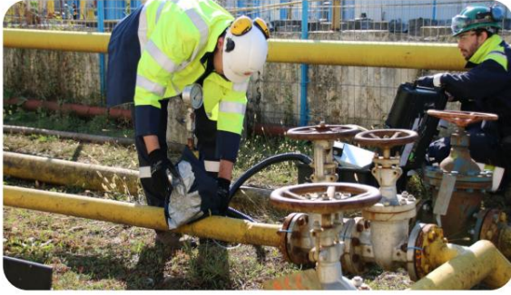
Figure 2. The Sniffers team scanning a site with an infrared camera (right panel) and deploying the HiFlow sampler on a leak (left panel) (Fotos: The Sniffers 2022)
