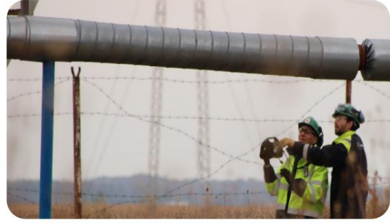
Figure 2. The Sniffers team scanning a site with an infrared camera (right panel) and deploying the HiFlow sampler on a leak (left panel) (Fotos: The Sniffers 2022)
