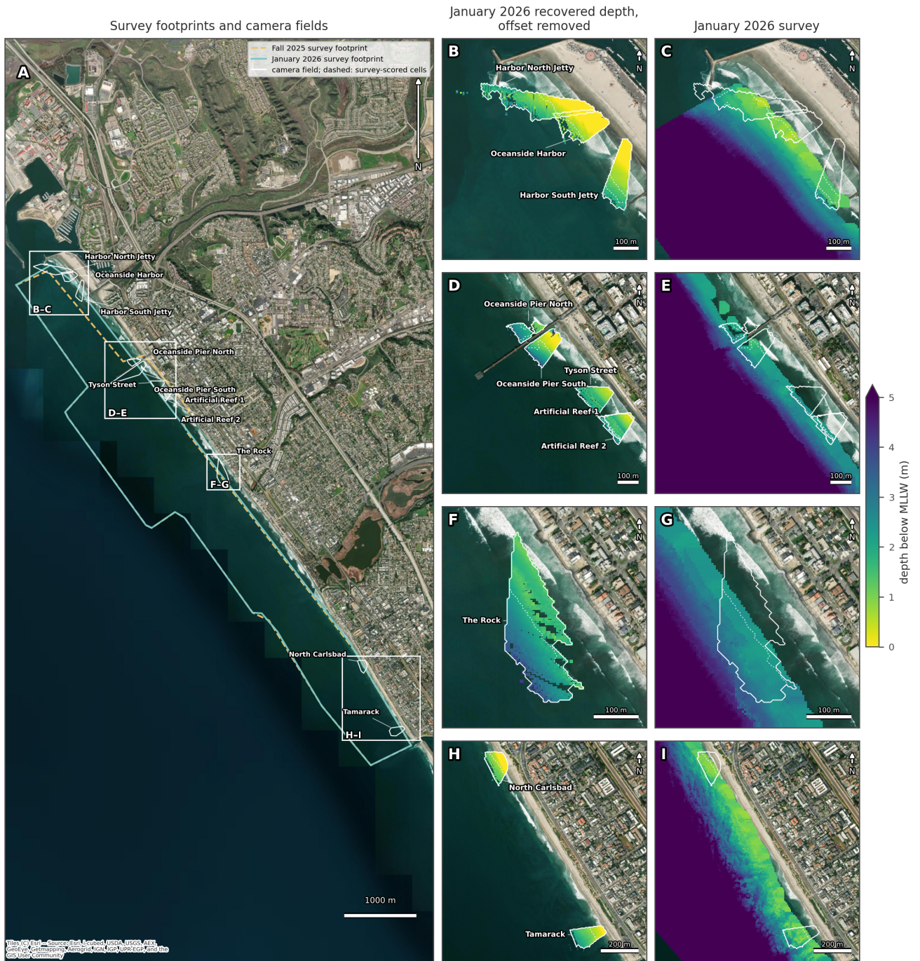
Figure 2: Survey footprints, camera fields and recovered depth. (A) Location map of the eleven cameras around Oceanside over satellite imagery, with the simplified footprints of the Fall-2025 survey (dashed amber) and the January-2026 survey (solid teal), which share their offshore edge, each camera's field outline and name, a north arrow and a 1000 m scale bar. White boxes mark the zoom panels. (B–I) January-2026 zooms on four camera clusters, from north to south Oceanside Harbor (B, C), Oceanside Pier to the artificial reefs (D, E), The Rock (F, G) and North Carlsbad and Tamarack (H, I), each with a north arrow and scale bar. The left panel of each pair shows the depth recovered on the 14-day window before the survey, with each camera's mean offset to the survey removed, and the right panel the survey depth over the same area, on one scale from 0 to 5 m below MLLW. The offsets are listed in Table 1; for Artificial Reef 1 it is taken from its 49 overlapping cells. White outlines trace each camera's field and dashed inner outlines the cells scored against the survey. The Fall-2025 results are in Table 1 and Fig. 4. Imagery © Esri. The figure places the cameras on the two surveys and lets the spatial pattern of each recovered field be compared with the survey beneath it.
