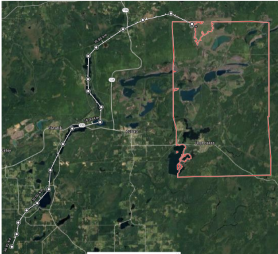
Figure 7: The main route of the simulated mud flow. After roughly 1.5 days, the mud from tailings dam breach travels roughly 36km along the lakes surrounding the dam
