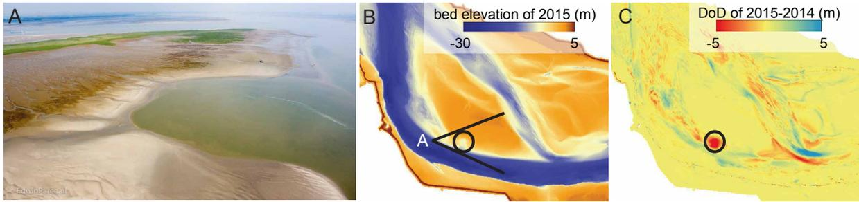
Figure 1: Example of a shoal margin collapse in the Western Scheldt Estuary. A) Aerial view of the tidal flat of Walsoorden after the July 2014 collapse (photo courtesy Edwin Parez, RWS). B) Bathymetry data ('vakkodingen') from the tidal flat of Walsoorden for 2015. C) Example DEM of Difference (DoD) between consecutive years used to identify location, geometry and shape of shoal margin collapses, here for the case shown in A and B.
