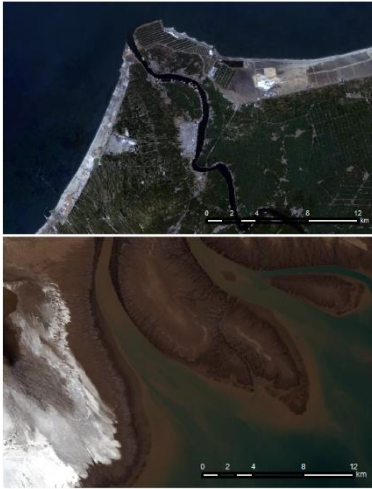
Fig. 3: (a) a natural color Landsat 8 image of the wave-dominated Nile river delta, where a clear distinction between land and water exists (b) a natural color Landsat 8 image of the tide-dominated Colorado river delta. The muddy intertidal flats and sediment plumes surrounding the mouth bars at the river mouth make high-accuracy shoreline extractions challenging.
