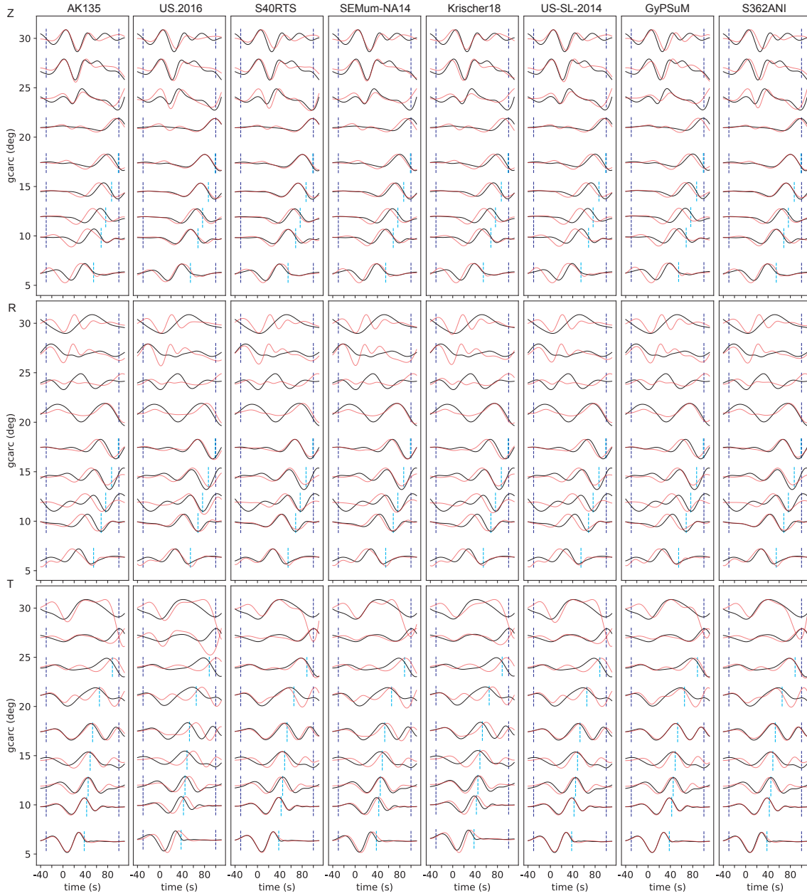
Figure A1. Waveform comparison for long period shear wave. The seismic recordings are filtered between 40–120 s and aligned with the theoretical arrival time of S-wave. Black and red lines are the observed and synthetic waveforms, respectively. Blue dashed lines mark the shear wave measurement window. Cyan dashed line indicates the starting of surface wave calculated by empirical surface wave speeds in Table. 2. Models S40RTS, S362ANI, US-SL-2014, and SEMum-NA14 have Crust1.0 on top.
