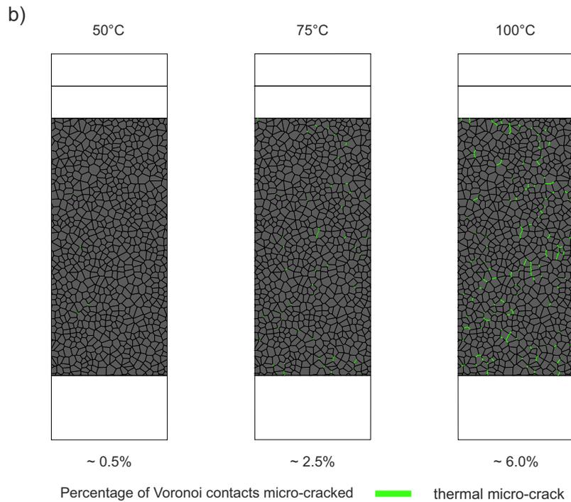
Figure 10: a) A subset of a numerical simulation thermally loaded to 100 °C showing  $x$ -component stresses ( $\sigma_{xx}$ ). The left hand edge of the subset is the edge of the model. Negative stresses are compressive. b) The amount of thermally induced micro-crack development in numerical simulations thermally loaded to 50 °C, 75 °C and 100 °C.
