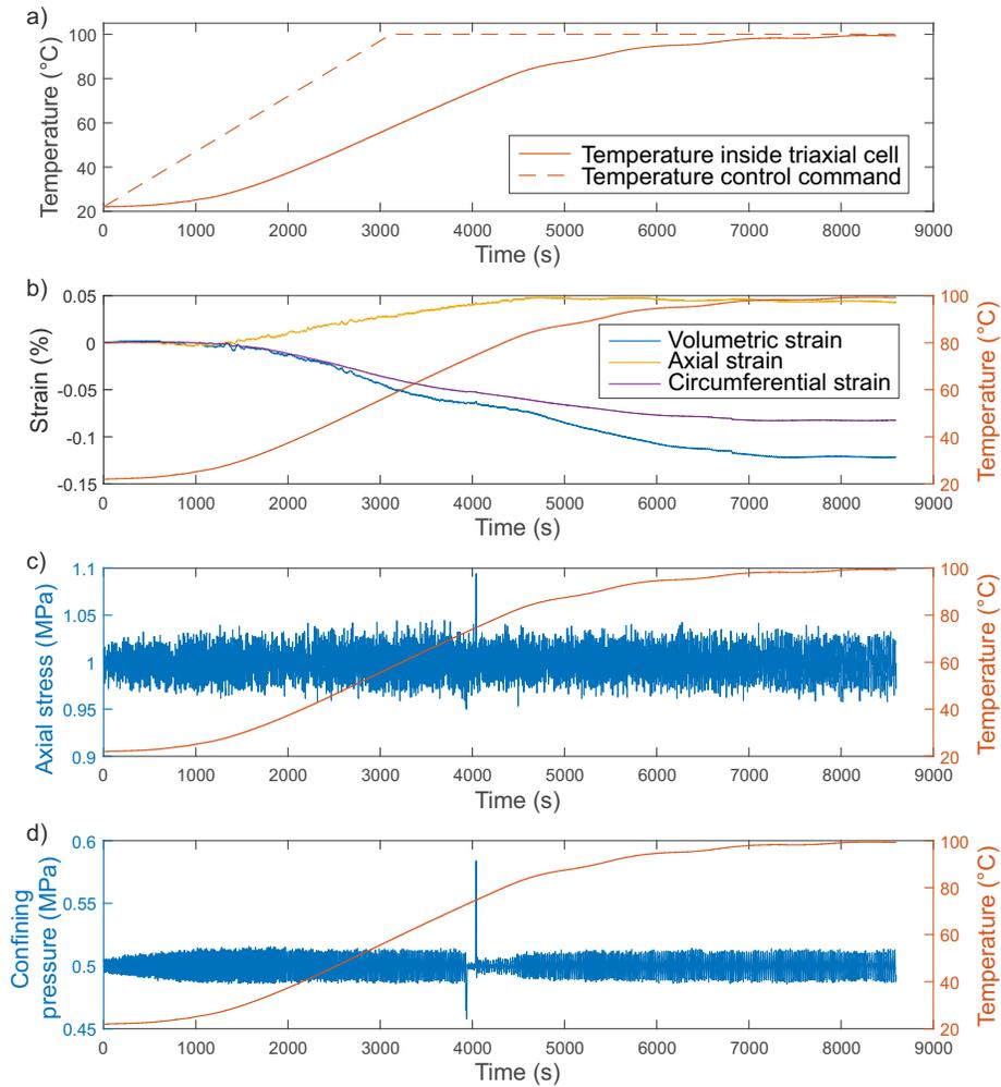
Figure 2: a) Thermocouple data on the heating of Specimen # 562 within the triaxial pressure vessel, compared with the  $1.5\text{ }^{\circ}\text{C min}^{-1}$  heating command. b) Volumetric, axial and circumferential deformation of the specimen during heating due to thermal expansion. c) Constant axial stress of 1 MPa maintained during thermal loading. d) Constant confining pressure of 0.5 MPa maintained during thermal loading.
