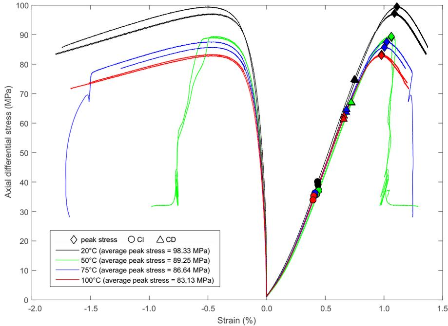
Figure 3: Axial stress vs. radial and axial strain data for triaxial tests on specimens of Thornhill Rock, carried out at 5 MPa  $\sigma_3$  and temperatures of 20 °C, 50 °C, 75 °C and 100 °C. (CI = crack initiation. CD = crack damage).
