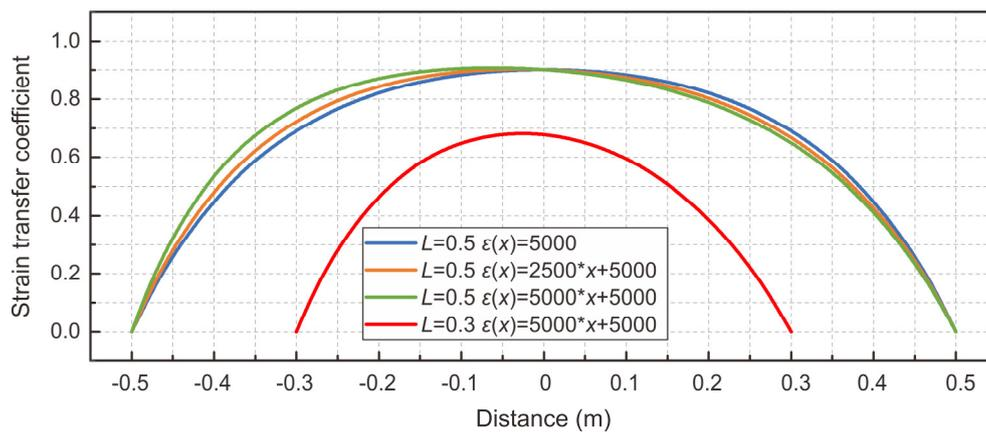
**Fig. 3.** Influence of bonding length and strain gradient on the strain transfer coefficient.
