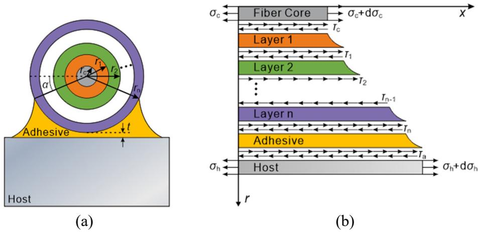
**Fig. 1.** Strain transfer analysis of surface-bonded multi-layered FO sensor. (a) Cross section. (b) Stress states of multi-layers.
