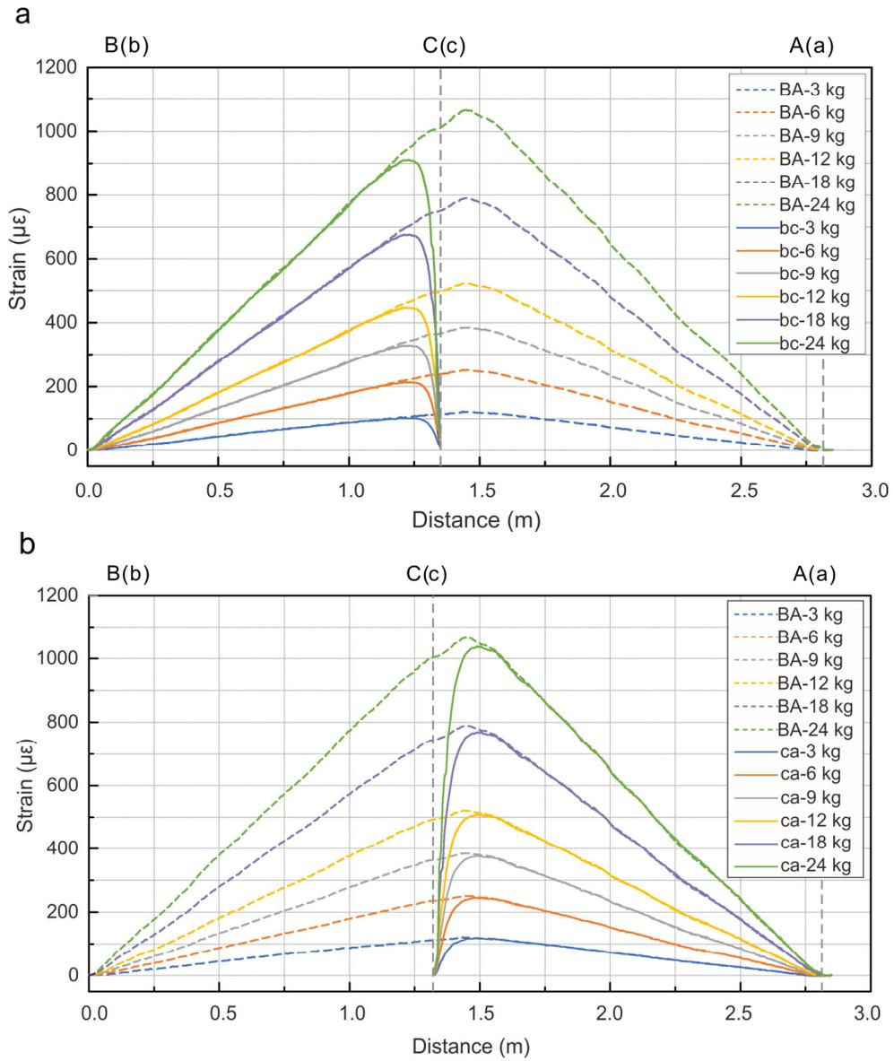
**Fig. 12.** Comparison of the strain distributions between cables AB and ab.
