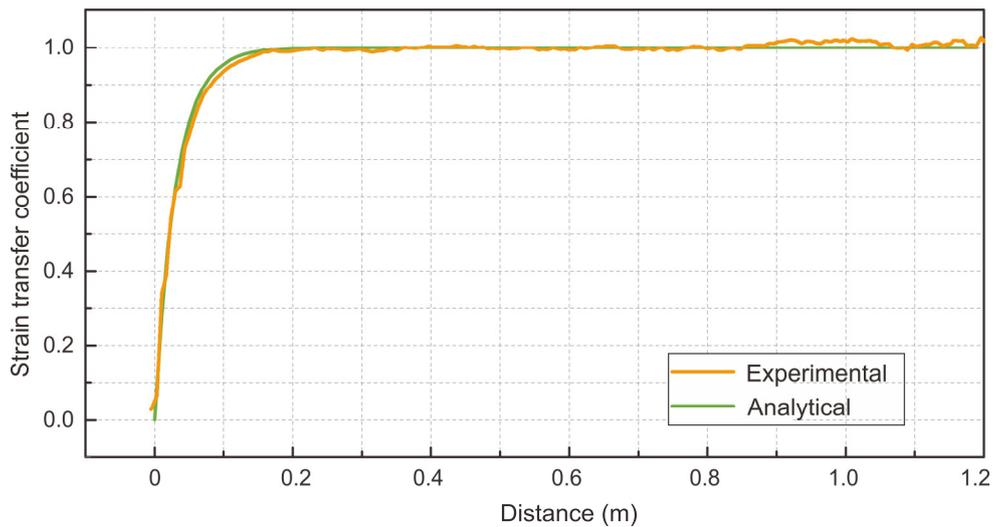
**Fig. 14.** Comparison between the experimental and theoretical strain transfer coefficients of cable ac.
