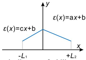
**Fig. 4.** Schematic diagram of a bilinear gradient strain.
