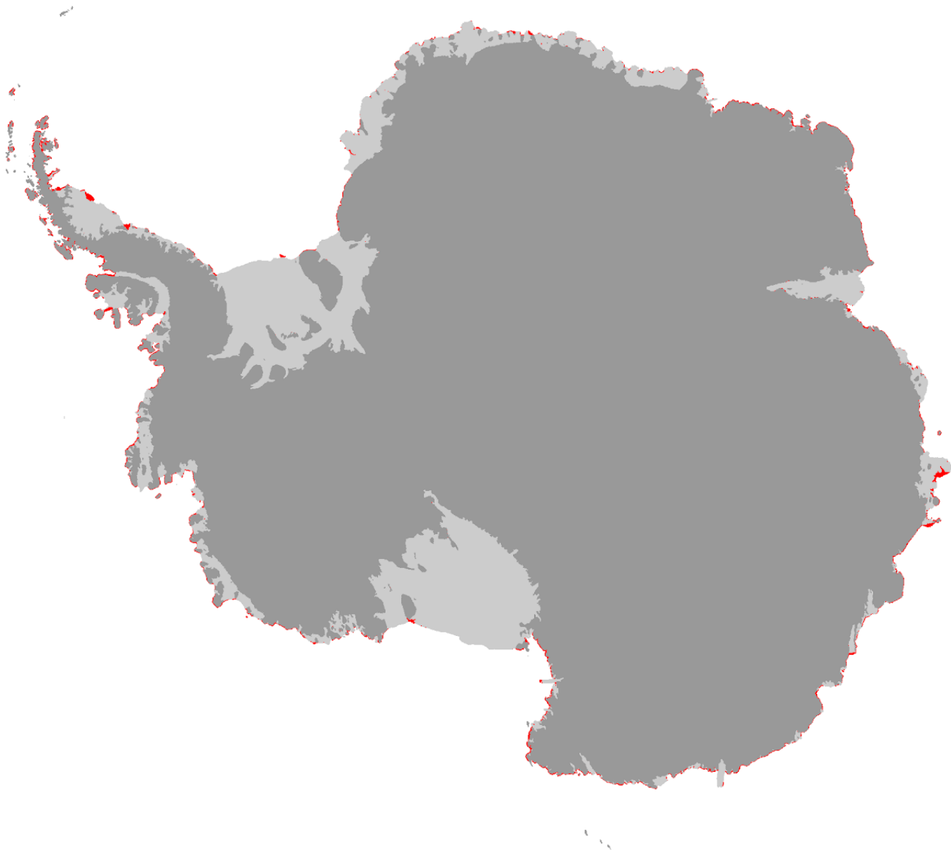
Figure B1. Difference in ice area definition. Red areas show ice that is excluded when imposing ice shelf boundaries from the MEaSURES Antarctic Boundaries data set (Mouginot et al., 2016) onto the ice draft from Bedmap2 (Fretwell et al., 2013).
