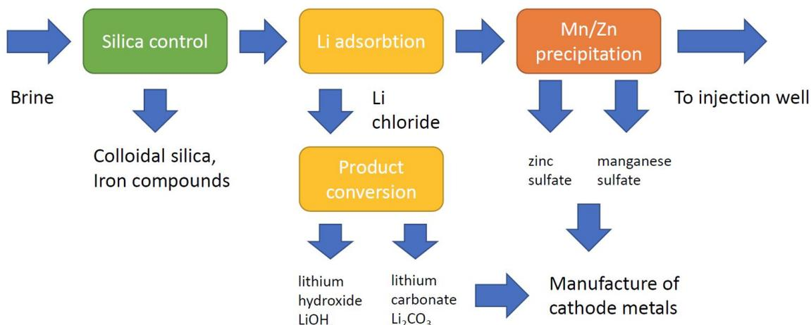
**Figure 7.4.** Scheme for extracting lithium and other valuable chemicals from Salton Sea geothermal brines. Mn/Zn removal can precede that of Li. Adapted from Harrison (2010a).
