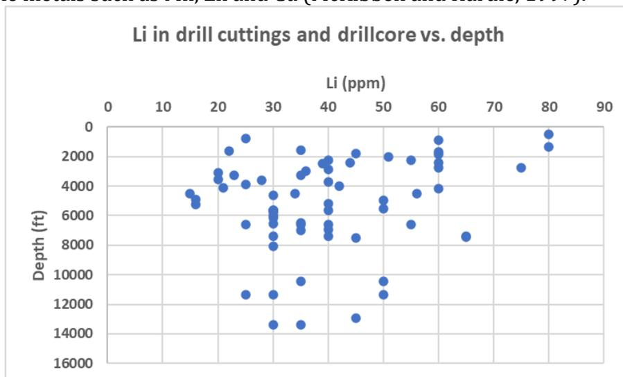
**Figure 7.3.** Variation of lithium (Li) metal content (in parts per million) versus depth for cuttings and core from several drill holes in the Salton Sea Geothermal Field. Based on
