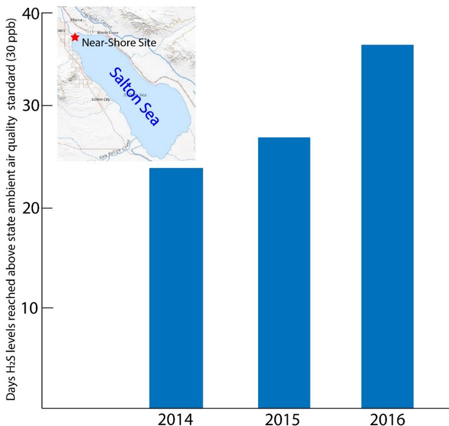
**Figure 3.2.** The number of days in the years 2014-2016 when hydrogen sulfide (H<sub>2</sub>S) levels surpassed state ambient air quality standard of 30 ppb at the Near-Shore air quality monitoring station near the Salton Sea (inset). These events are linked to hydrogen sulfide production in the lake and regional wind patterns and result in widely distributed 'rotten egg' odors during the summer. Data from the public records of the South Coast Air Quality Management District.
