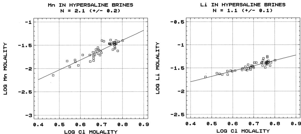
**Figure 7.2.** Variation of dissolved manganese (Mn) and lithium (Li) metal content (in molality: moles of metal per kilogram of brine) as a function of the brine’s chlorinity (dissolved chlorine molality) in the Salton Sea Geothermal Field reservoir brines. Adapted from McKibben and Williams, 1989, including unpublished data on lithium).
