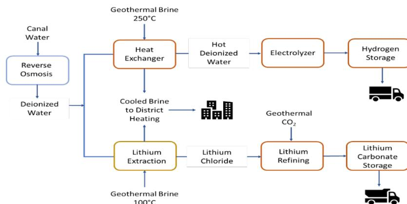
**Figure 7.6.** Conceptual design of lithium and hydrogen extraction from Salton Sea geothermal brines at temperatures of 250° and 100°C. From Elders et al., 2019. Direct conversion of Li chloride to a Li hydroxide product would be more advantageous for battery manufacture.
