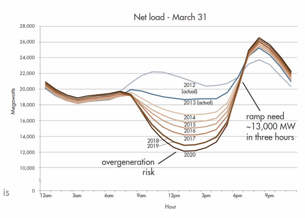
**Figure 7.5.** Projected daily electricity demand, minus wind and solar generation, on a typical spring day in California. There is a risk of overgeneration in the middle of the day and early afternoon, followed by a steep ramp where an additional 13 GWe is needed (Source: California Energy Commission, 2017, Figure ES-4).
