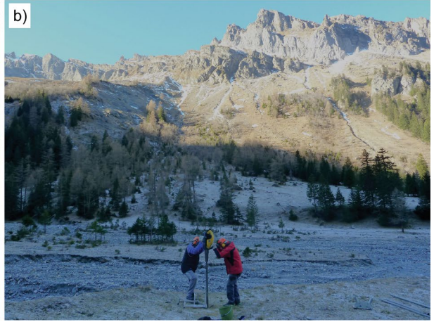
Figure S1. Photographs showing a) the concrete weir gauging station S2, and b) the installation of piezometer N4.
