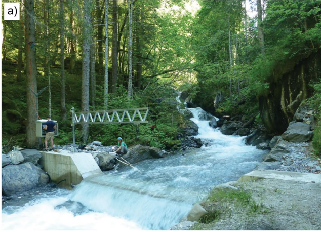
Figure S1. Photographs showing a) the concrete weir gauging station S2, and b) the installation of piezometer N4.
