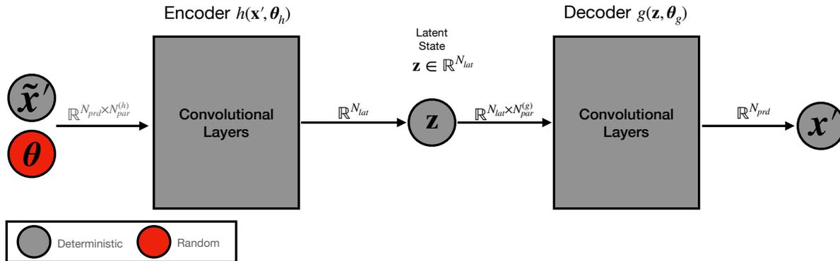
**Fig. 7** A diagram of the convolutional architecture of the deterministic autoencoder (10).
