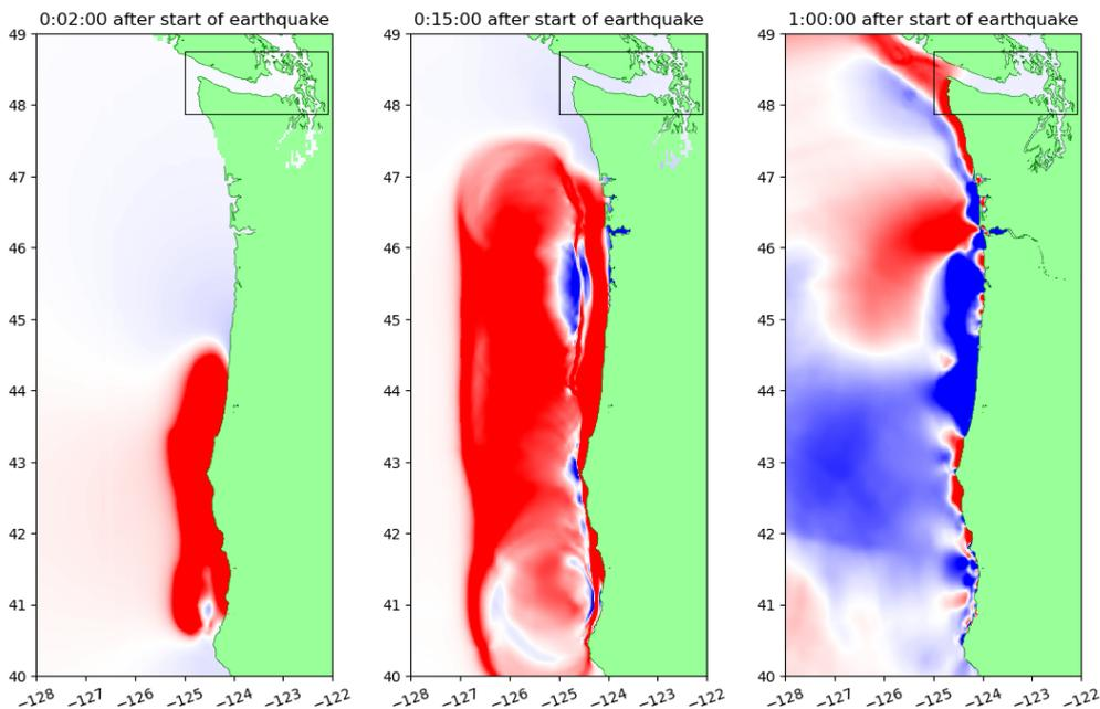
**Fig. 3** Tsunami from Realization #1127 at times 0:02, 0:15 and 1:00. Colors show surface elevation and saturate at  $-0.5\text{m}$  (blue) and  $+0.5\text{m}$  (red). Note that at time 0:02 the sea floor deformation is still in progress. For this realization, the earthquake ruptures from south to north with a total duration of about 4 minutes.
