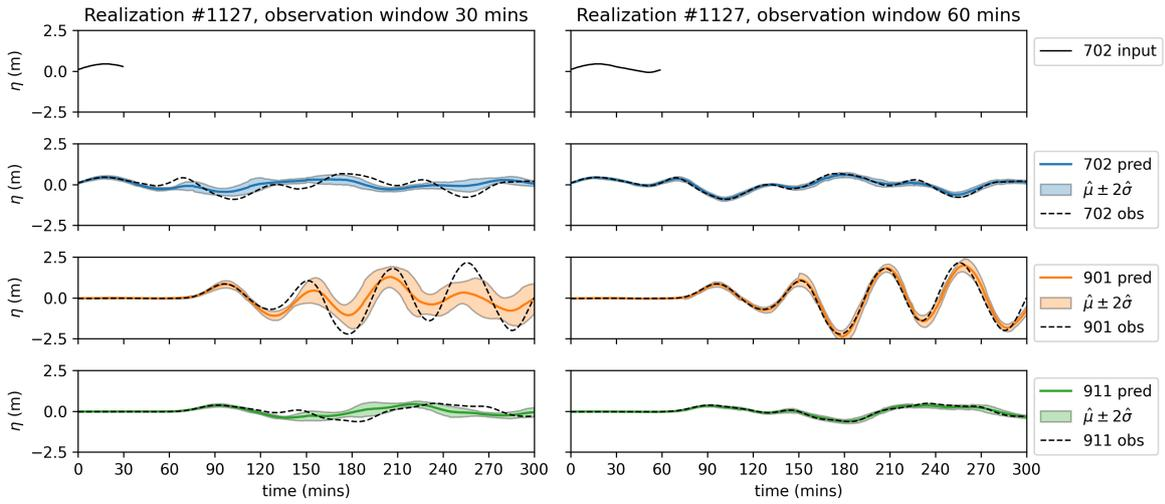
**Fig. 11** Predicted time series for realization #1127 using the DAE, based on the observed data shown in the top row for observation window 30 minutes (left column) or 60 minutes (right column). The sensitivity of the model to the initial guess for the parameters is indicated by the uncertainty bands, as described in the text.
