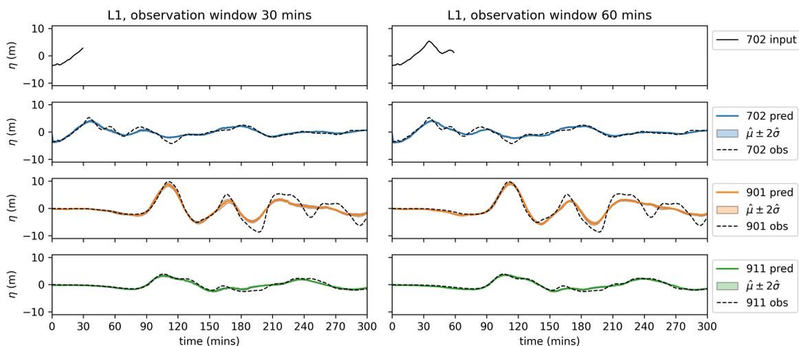
**Fig. 17** Predicted time series for the L1 scenario using the VAE, based on the observed data shown in the top row for observation window 30 minutes (left column) or 60 minutes (right column).
