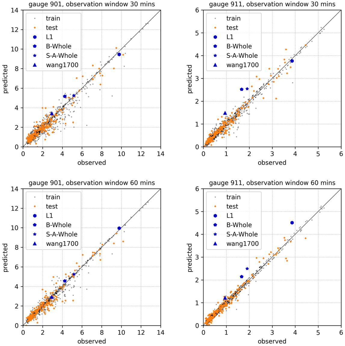
**Fig. 6** Prediction results using the SVM at gauge 901 (left column) and 911 (right column). Prediction results are compared when using an observation window  $T_{ow} = 30$  minutes of time series data (top row) and 60 minutes of time series data (bottom row). In each case the scatter plot shows the predicted maximum tsunami elevation vs. the observed maximum from the full simulation, with one point for each realization tested.
