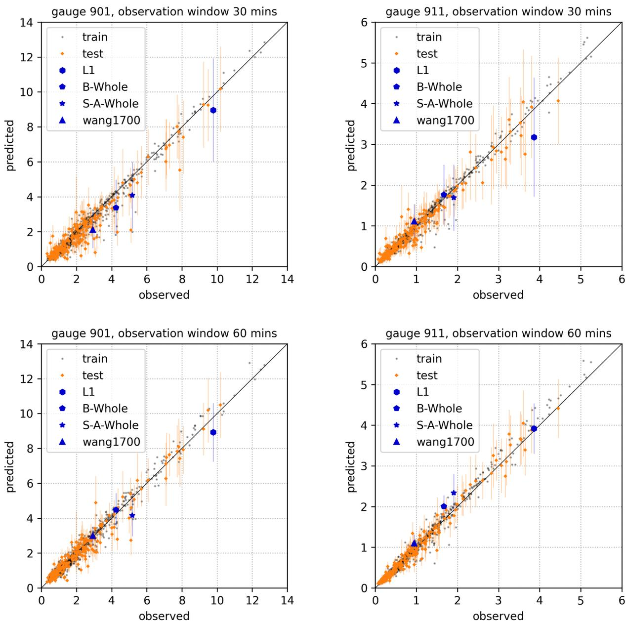
**Fig. 9** Prediction results using the DAE, as explained in the caption of Figure 6, with the addition of a vertical bar centered on each test prediction showing  $2\sigma$  for the uncertainty in the prediction, as explained in Section 5.
