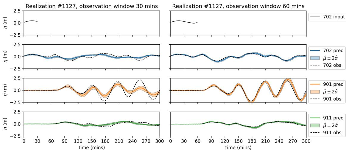
**Fig. 16** Predicted time series for Realization #1127 using the VAE, based on the observed data shown in the top row for observation window 30 minutes (left column) or 60 minutes (right column).
