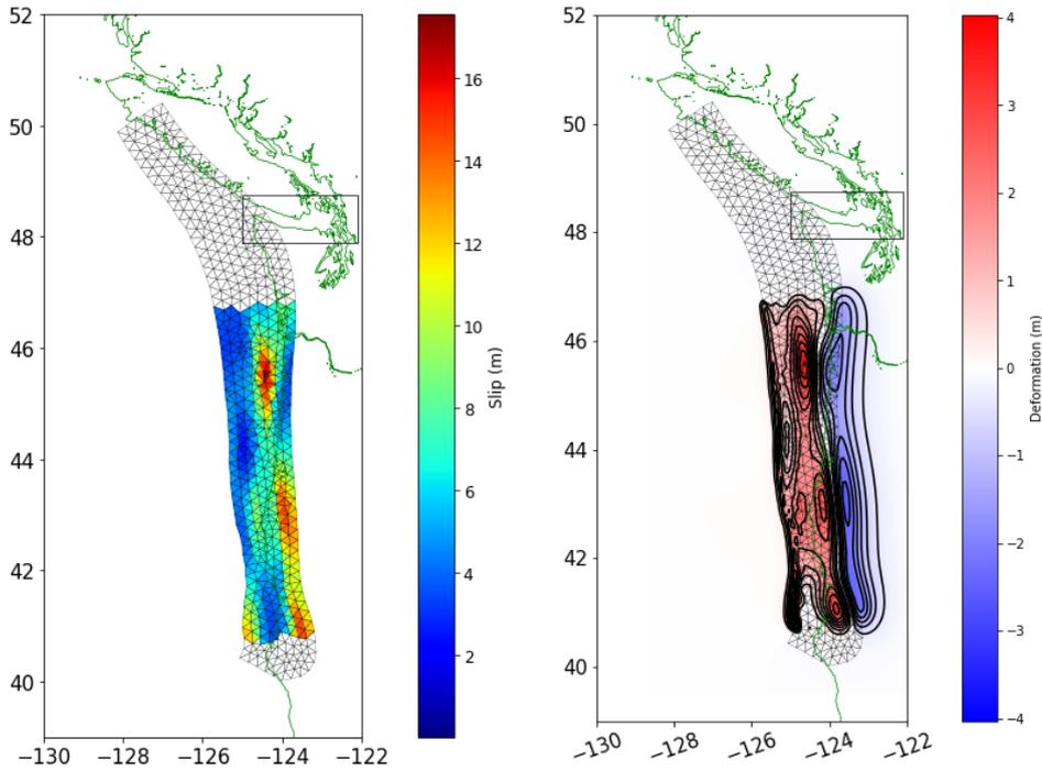
**Fig. 1** Left: Surface projection of the triangular subfaults of Slab 1.0 model of CSZ together with slip from a sample realization #1127, with Mw 8.8. Right: Final seafloor deformation for realization #1127 as computed with the Okada model. In each figure, the black rectangle shows the SJDf region that is shown in more detail in Figure 2.
