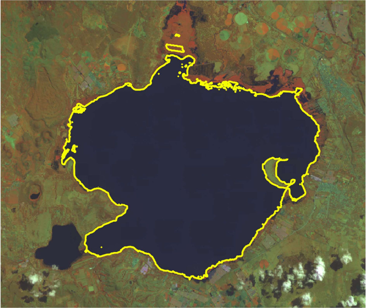
1470 Figure A7: Land-water mask indicated by yellow polygons for Lake Naivasha for 20.07.2020
