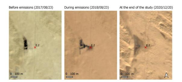
**Fig. S3.** The evolution of the E.2 emission point seen in RGB before, during and after the emissions derived from a leak. During the emission period a black liquid emanating from the emission point
