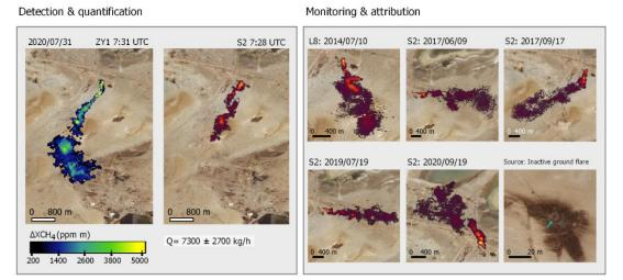
**Figure 3.** Examples of emissions detected from the A.3 emission point (see Fig. 2). Left, plume detected by both ZY1 and S2 within a 3-minute time difference. Right, time series of plumes detected at A.3 with the S2 and L8 multispectral satellites. A true-color composite of the emission point, based on visual imagery, is shown in the lower right corner. The background image for all panels is from Bing Aerial.
