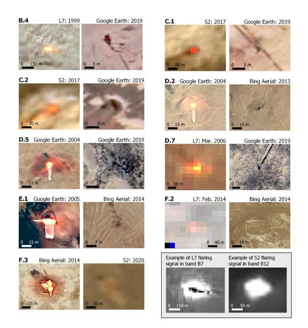
Fig. S1. Flares with active flaring in the past and current inactive appearance seen in RGB. Bottom right two examples of active flares as seen in the Landsat 7 (L7) B7 and S2 B12 bands (points D.7 and C.2 respectively), i.e. in the CH4 absorption bands. In the Landsat B7 and S2 B12 bands, the CH4 absorbs the signal (low values), while the flaring emits a very high signal (very high values) compared to the surface.
