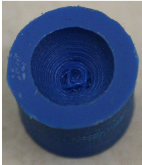
Figure 2. Visualisation of the printing quality of the top of the spherical void of the hollow cylinder. Only the top half of the hollow cylinder was printed for visualisation purposes and the sample is displayed upside down.
