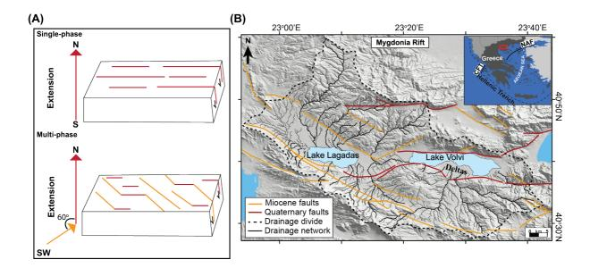
**Figure 1. (a)** Block diagrams showing the structural set-up used in this study to simulate the evolution of rift basins under single and multi-phase rifting and **(b)** hillshade map of the Mygdonia Rift (northern Greece) that has experienced two phases of non-coaxial extension; a NE-SW extension during the Miocene and a N-S extension during the Quaternary.
