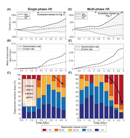
**Figure 4.** Time evolution plots showing maximum, minimum and mean elevation (in m) in (a) and (d), and mean erosion and sedimentation rates (in mm/yr) in (b) and (e), at 0.5 Myr intervals for the single-phase and the multi-phase rift experiments, respectively. Percentage of depocentre surface area (%) over the total model domain is shown for different sized depocenters (in km<sup>3</sup>) in (c) for the single-phase experiment and in (f) for the multi-phase experiment.
