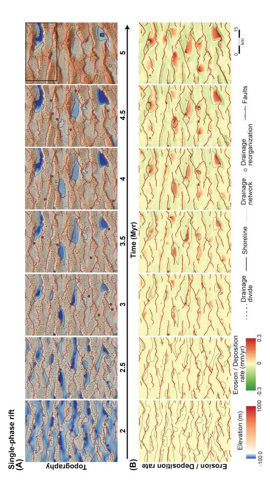
**Figure 3.** Modelling results showing (a) topographic and (b) erosion and deposition rate evolution from 2 Myr to 5 Myr, at 0.5 Myr intervals, for the single-phase rift experiment. In (a), red stars depict drainage integration events and yellow stars depict drainage isolation. Black box at 5 Myr shows a part of the model area that is illustrated in 3D in Fig. 5 and capital letter '**B**' marks the basin shown in inset in Fig. 10b.
