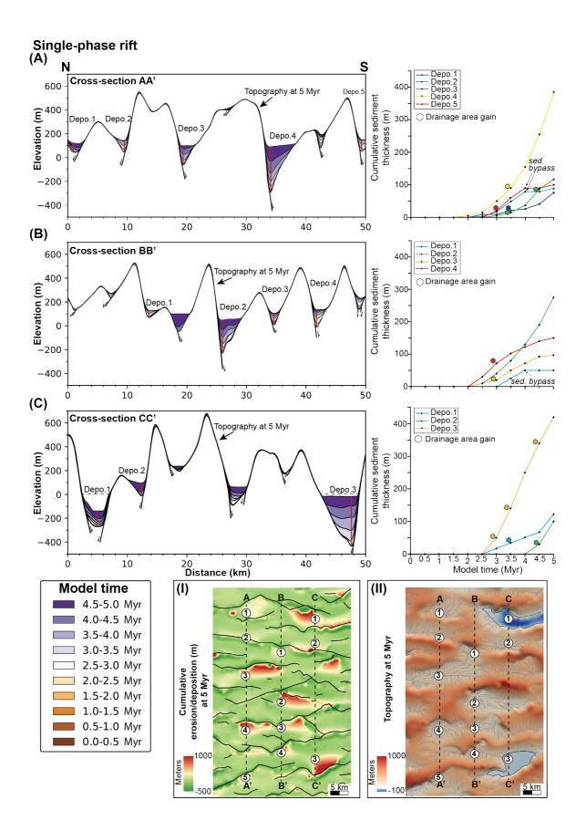
Figure 6. Cross sections (a) AA', (b) BB' and (c) CC' in N-S direction showing stratigraphic
