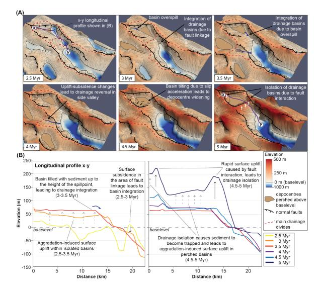
Figure 5. (a) Topographic evolution in 3D from 2.5 Myr to 5 Myr for part of the single-phase rift experiment (for location see Fig. 3a) showing examples of drainage integration due to basin overspill and fault linkage and examples of drainage isolation in response to fault interaction.(b) x-y longitudinal profile crossing through the basins shown in (a) for the same time period.
