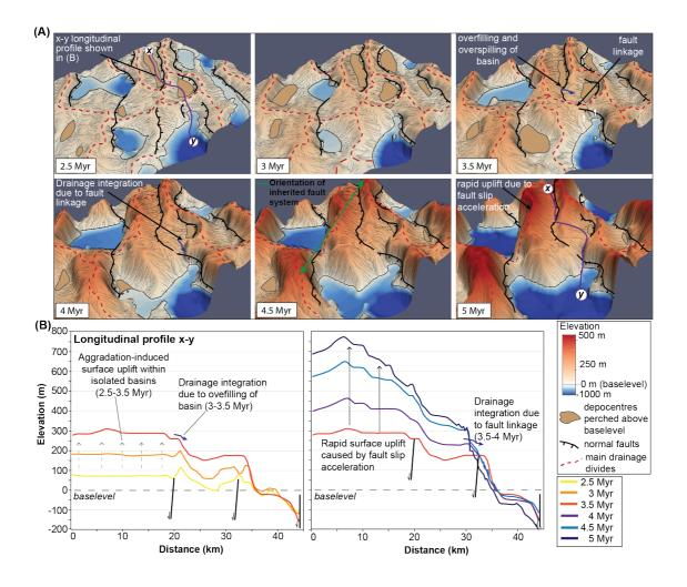
Figure 8. (a) Topographic evolution in 3D from 2.5 Myr to 5 Myr for part of the multi-phase rift experiment (for location see Fig. 7a) showing examples of drainage integration due to basin overspill and fault linkage and examples of drainage isolation in response to fault interaction.
