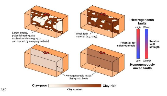
Figure 4 Schematic fault model showing the effect of heterogeneity on fault strength and stability.
