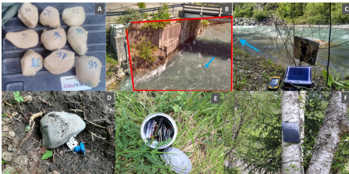
221 222 Figure 2. RFID devices, geophone station (A: artificial tracers equipped with a-UHF tags; B: the e-RFIDuino 223 station; C: the mobile station RFID 1) and geophone datalogger (D: the Geospace ® GS-20DX geophone before 224 its installation on a rock; E: the encapsulated datalogger of the geophone signal; R: solar panel).
