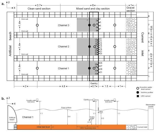
Figure 1. (a) Plan view and (b) Side view of the experimental set-up. The grey area is scanned by an Ultrasonic Range System (URS) with numbered sensors (black squares). White and black circles denote acoustic water level sensors and Vectrino profilers, respectively. Dimensions are in metres.
